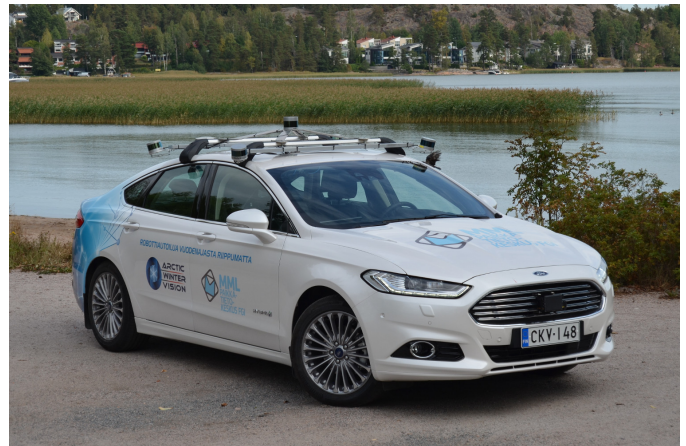
Fig. 1. FGI autonomous driving research platform ARVO.
