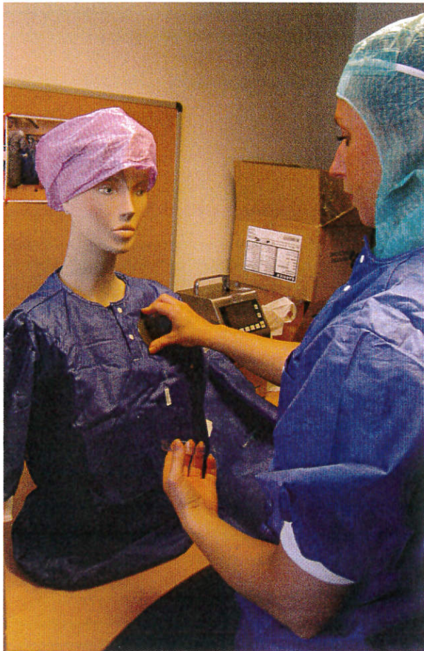
Figure 3. Contact sampling performed on the surgical clothing system of the test dummy. (Photo B, Reinmüller in Jordstedt 12 ).
