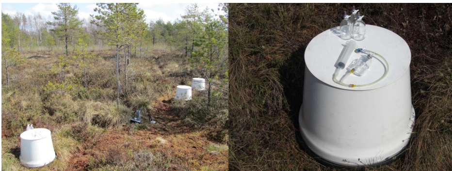
Figure 6. Sampling plot on a study transect in Estonian transitional mire (left), closed static chamber on a collar for GHG sampling (right). Photos by Gert Veber.
