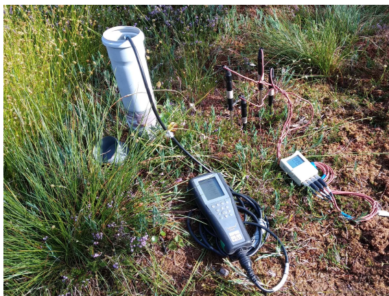
Figure 7. Water level observation and sampling well with YSI Water Quality Instrument and soil temperature logger. Photo by Gert Veber.
