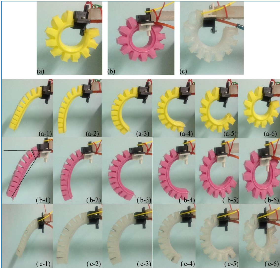
Figure 8. experimental results of single actuator under different air pressure: (a) full bending of actuator fabricated with RTV 4503, (b) full bending of actuator fabricated with RTV 225 , (c) full bending of actuator fabricated with Elastosil M4600, (a-1, b-1, c-1) actuators at 0 kPa (Initial position) , (a-2, b-2, c-2) actuators at 10kPa , (a-3, b-3, c-3) actuators at 20kPa, (a-4, b-4, c-4) actuators at 30kPa, (a-5, b-5, c-5) actuators at 40kPa (a-6) actuator fabricated with RTV 4503 bending at 51kPa, (b-6) actuator fabricated with RTV 225 bending at 48kPa, (c-6) actuator fabricated with Elastosil M4600 bending at 58kPa.
