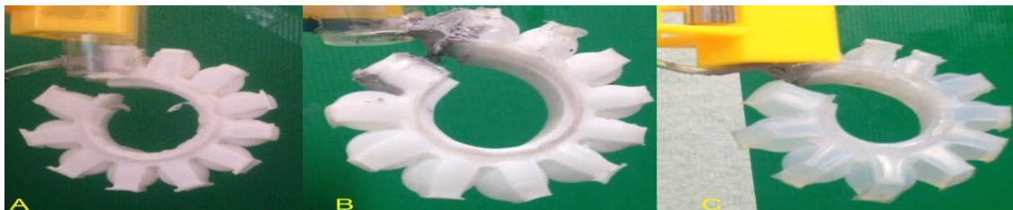
Figure 7. Bending at 360 degree (A) Silicon RTV 4503 actuator full bending at 85 KPa (B) Silicon RV 225 actuator full bending at 75 KPa (C) Silicon Elastosil M4600 actuator full bending at 90 KPa.
