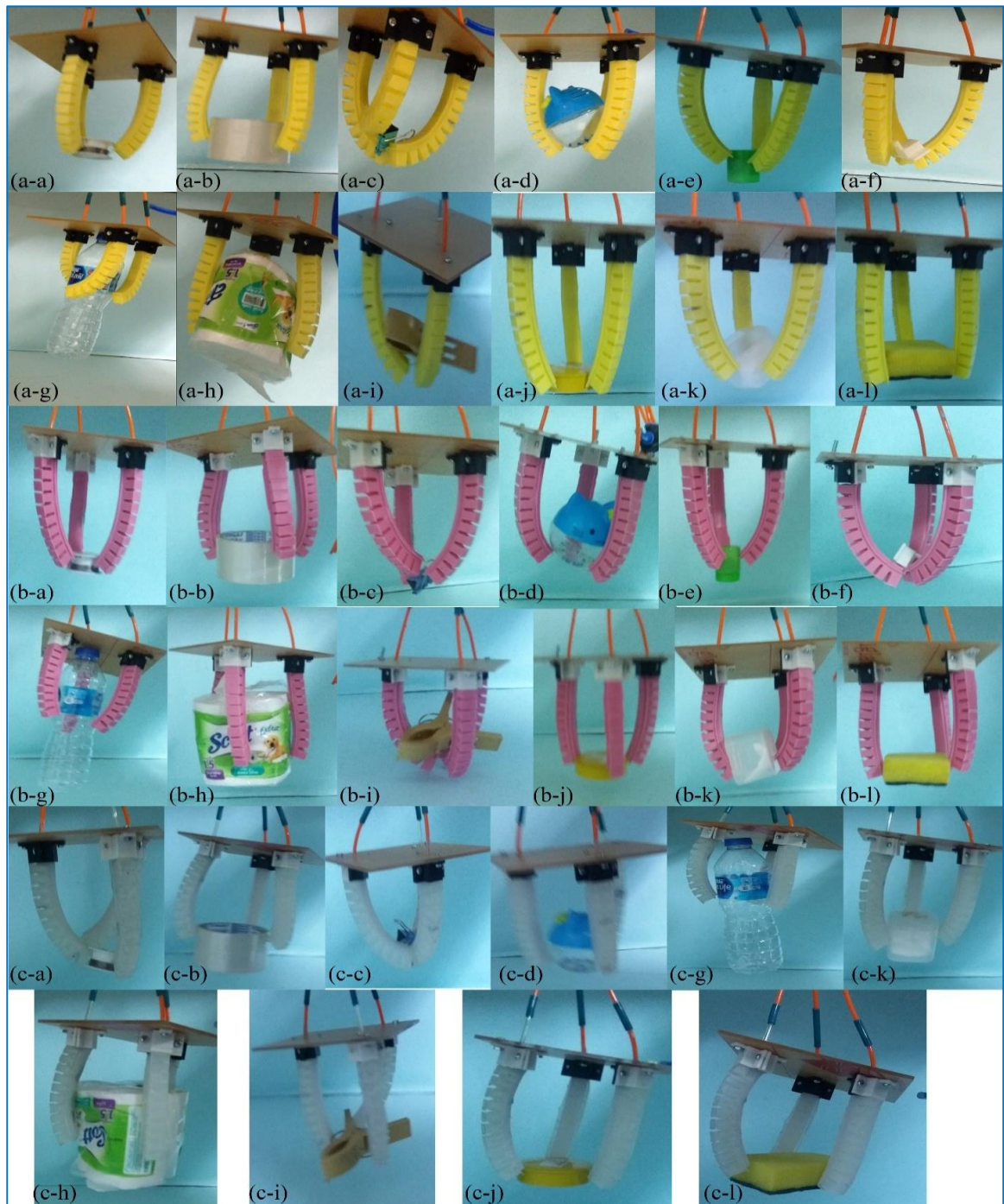
Figure 12. Grasping experiment with different objects using all three material actuator type.
