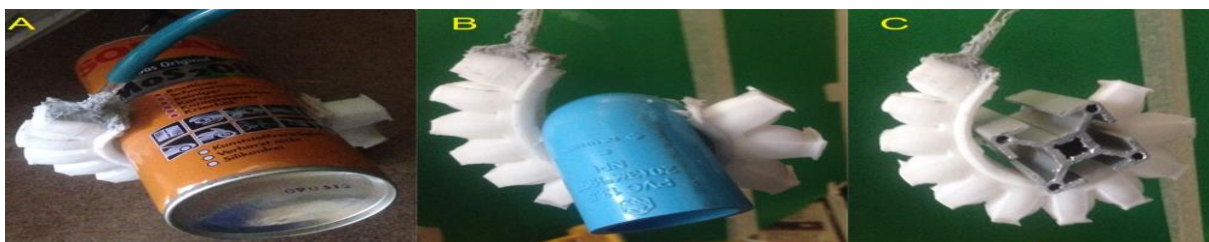
Figure 9. Grasping different object with RTV 4503 actuator (A) circular bottle (B) circular pipe (C) rectangular shape.
