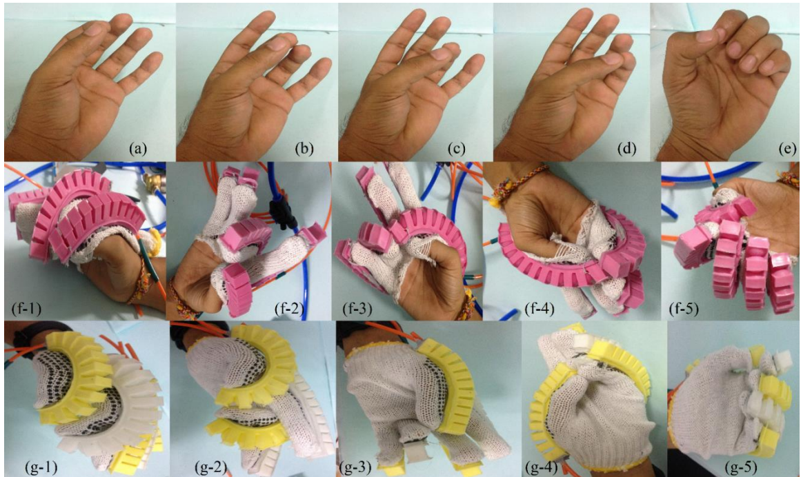
Figure 11. Kapandji test for rehabilitation purpose: (a) thumb contact with index finger (b) thumb contact with middle finger (c) thumb contact with ring finger (d) thumb contact with small finger (e) full hand flexion (f-1 – f-4) soft robotic glove assembled with RTV 225 performing all above posture (g-1 – g-4) robotic glove performing the human hand posture for rehabilitation standardized test.
