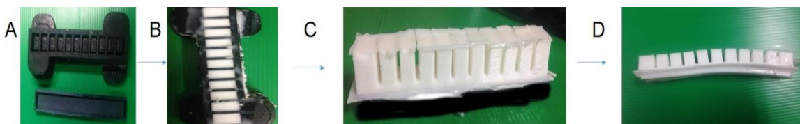
Figure 5. Overview of fabrication process (A) 3D printed molds (B) pouring of silicon in air chamber mold (C) Sealing the air chamber with base mold (D) fabricated air chamber with air inlet.
