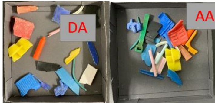
Figure 4.5: The two different arrangement of the samples, agglomerated arrangement AA and dispersed arrangement DA
