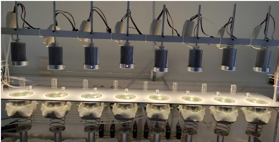
Figure 3. The JyrkkiII gas-exchange system. It consists of 8- cylindrical chambers, a glass on top of it covers the chamber, springs support the pots from the bottom to keep them steady, and lamps are used as light source. Plants were grown through a hole in a glass, placed under the chamber to be measured for gas-exchange experiments.
