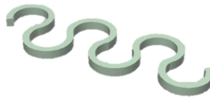
Figure 3.17 The “horseshoe” serpentine shape structure
