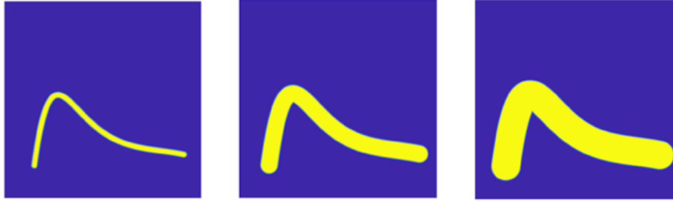
Figure 3.5 The Effect of parameter w on geometry mapping: (a) w = 1 , (b) w = 3 , and (c) w = 5 for \beta = 5
