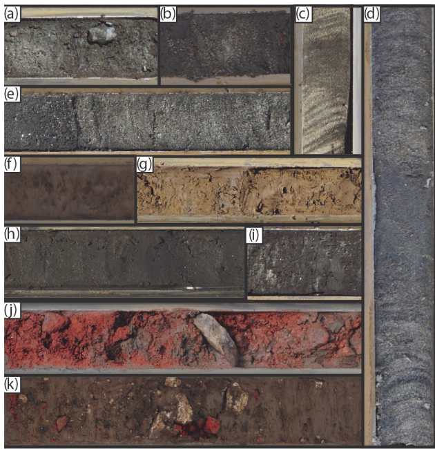
Figure 6. Exemplary core sediments corresponding to the different sedimentary units. Selected sediments of the coring material representing the identified units. (a, b) unit basement, (c) unit point bar, (d) unit levee, (e) unit riverbed, (f, g) unit reworked alluvium, (h, i) unit floodplain, (j) unit cultural debris, and (k) unit cultural environment.
