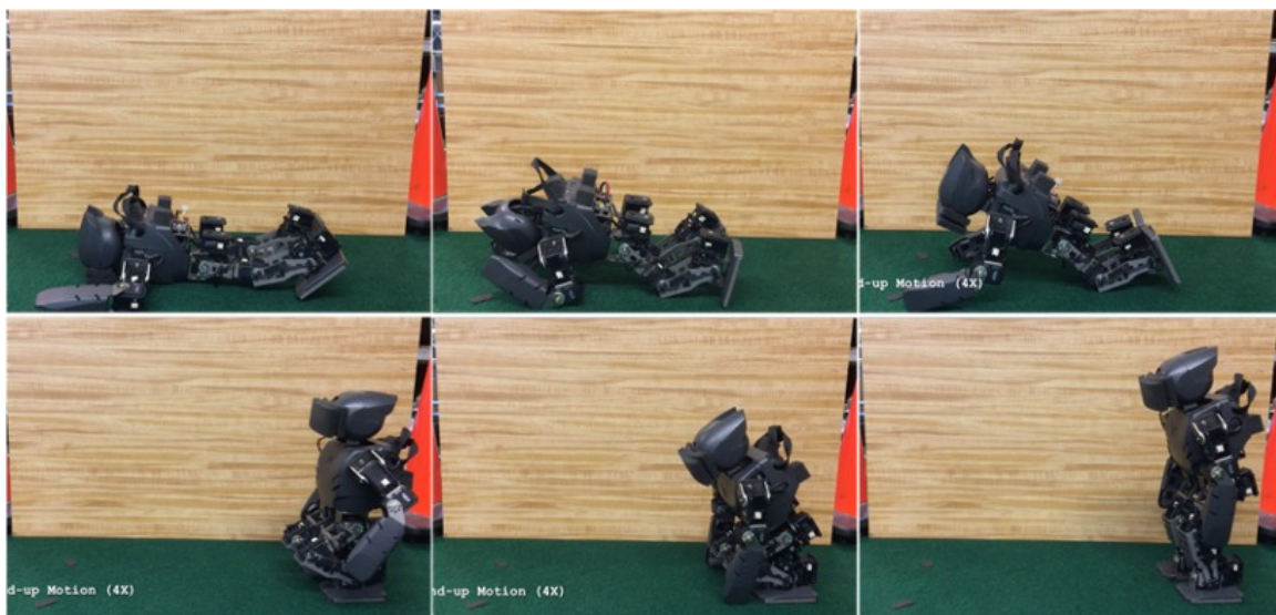
Figure 3.8: A sequence of a successful stand-up motion of a real-robot experiment example (from top left to bottom right).
