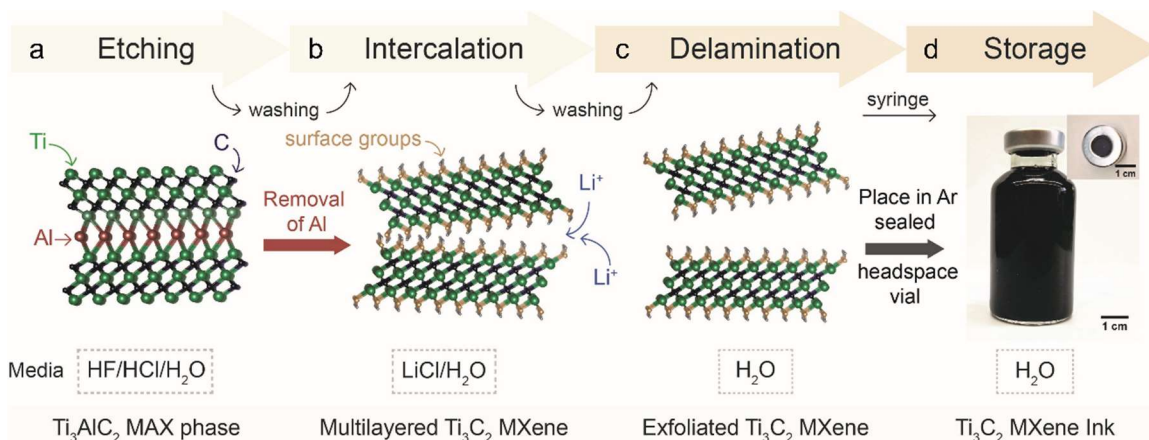
Figure 4.3 Schematic depicting MXene synthesis procedure. (a) \text{Ti}_3\text{AlC}_2 MAX is added to a selective etchant solution (HF, HCl, and DI \text{H}_2\text{O} ), resulting in the removal of aluminum (Al). (b) After washing the etching solution to neutral pH using DI \text{H}_2\text{O} , multilayered \text{Ti}_3\text{C}_2 is obtained. Multilayered \text{Ti}_3\text{C}_2 is intercalated with \text{Li}^+ from an aqueous solution of lithium chloride (LiCl). (c) After washing the intercalation reaction, sediment swelling is observed representing the exchange of \text{Li}^+ with \text{H}_2\text{O} . Agitation of the swollen sediment results in exfoliated (or delaminated) single- to few-layer flakes of \text{Ti}_3\text{C}_2 MXene in \text{H}_2\text{O} . Size selection and separation of delaminated \text{Ti}_3\text{C}_2 MXene from multilayered \text{Ti}_3\text{C}_2 and \text{Ti}_3\text{AlC}_2 MAX phase occurs at this stage. (d) \text{Ti}_3\text{C}_2 MXene ink is transferred via syringe to an Argon sealed headspace vial for long-term storage.
