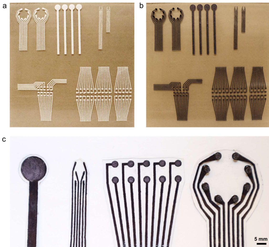
Figure 5.3 Scalable fabrication of MXtrode arrays. (a) Photo of laser-patterned array substrates for various device and array geometries. (b) The same batch of devices shown in (a) after infiltrating with MXene ink. In the top left are shown the EEG ring MXtrode arrays after addition of the 3D mini-pillars. (c) Photographs of completed devices (from left to right) designed for ECG, ECoG, EMG, and EEG sensing.
