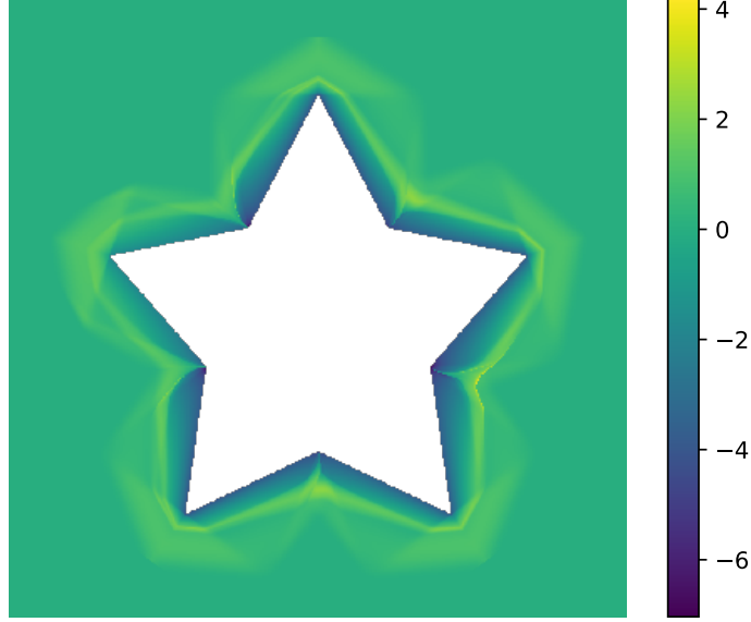
Figure 7.5: Values of \det(D_{\mathbf{x}}\mathbf{h}^{\mathcal{I}}) for a single polygon in logarithmic scale, showing the local nature of the diffeomorphism ( \mathbf{h}^{\mathcal{I}} becomes equal to the identity transform away from the polygon) and the fact that \mathbf{h}^{\mathcal{I}} is smooth away from sharp corners, that do not lie in the interior of the freespace.
