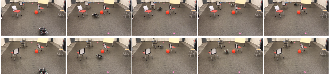
Figure 7.20: Snapshots of Minitaur avoiding multiple familiar obstacles in two different settings, using offboard perception.
