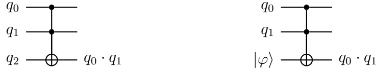
(a) Example circuit with an output qubit, q_2 (b) Example circuit with an output qubit labeled as |\varphi\rangle
