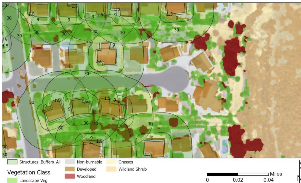
Figure 16 Buffer zones of increasing size (0 - 1.5 m, 1.5 m – 9 m and 9- 30 m) around houses included in the analysis.
