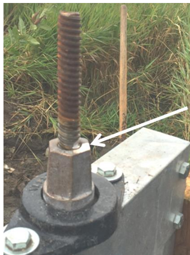
Figure 17. The "zero" opening mark ground into the threaded rod
