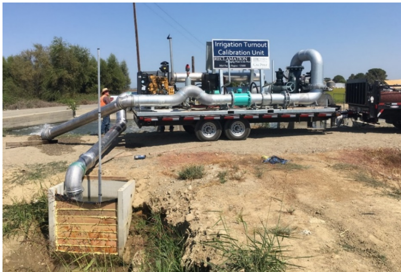
Figure 13. USBR/ITRC Irrigation Turnout Calibration Unit
