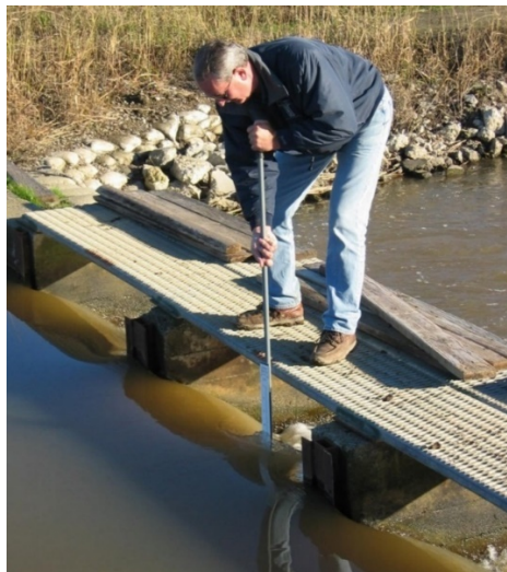
Figure 42. Use of an ITRC weir stick on flashboards
