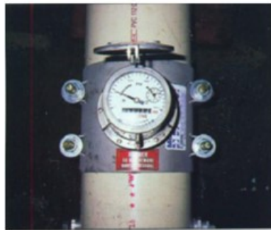
Above, propeller flow meter, the most common flow meter used for irrigation pumping plants. Below, flow meter installed in test section used for this study.
