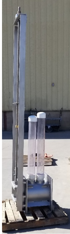
Figure 23. Side view of prefabricated canal metergate (Fresno ID, 2019)
