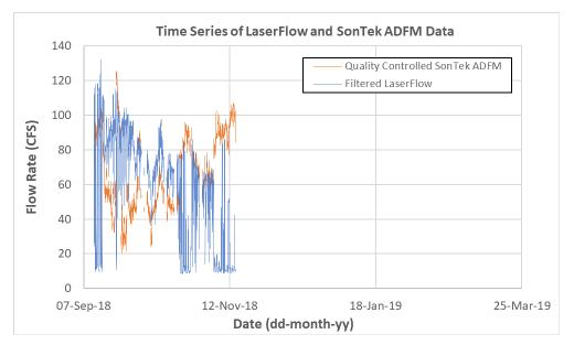
Figure 5. Hourly LaserFlow and SonTek ADFM flow rate data
