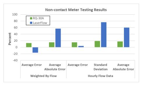
Figure 4. Results of non-contact meter testing at PID
