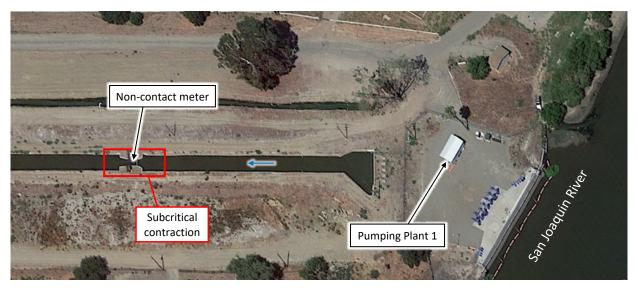
Figure 2. Aerial map view of PID Main Canal and non-contact meter installation
