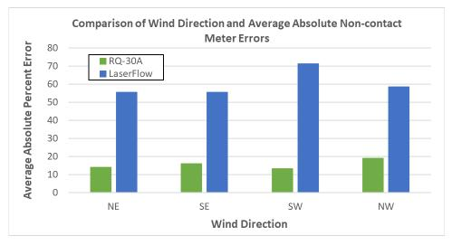
Figure 9. Non-contact meter average absolute percent errors for each wind direction
