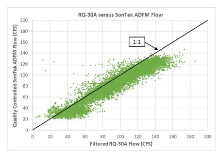
Figure 8. Comparison of filtered RQ-30A flow rate to quality controlled SonTek ADFM flow rate
