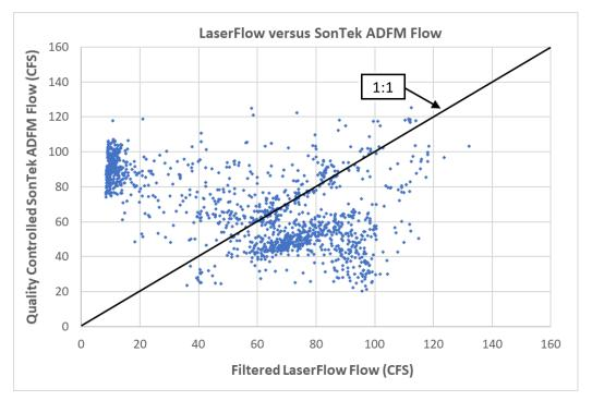
Figure 6. Comparison of filtered LaserFlow flow rate to quality controlled SonTek ADFM flow rate
