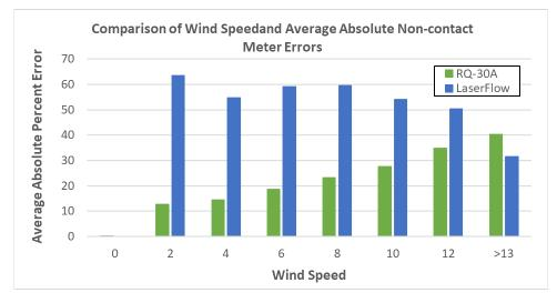
Figure 10. Non-contact meter average absolute percent errors for each wind speed
