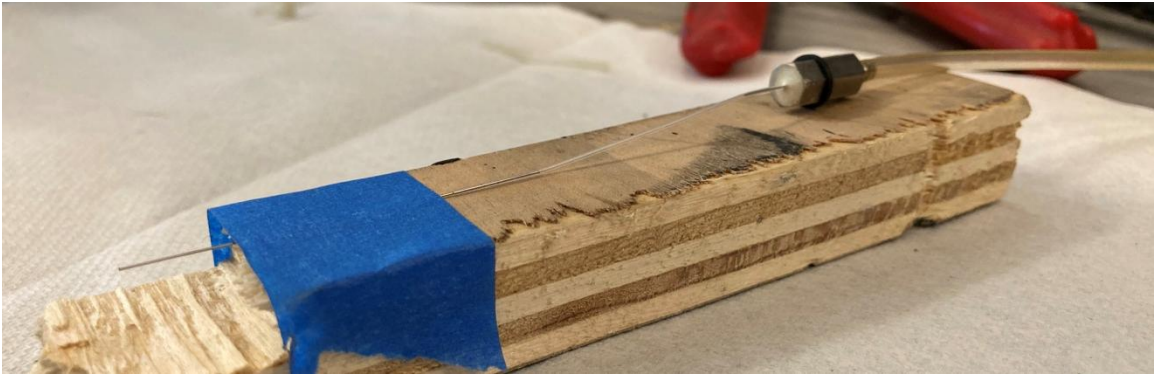
Figure 80: Tabletop Assembly Used to Flow Test the Internals of the Preston Tube.
