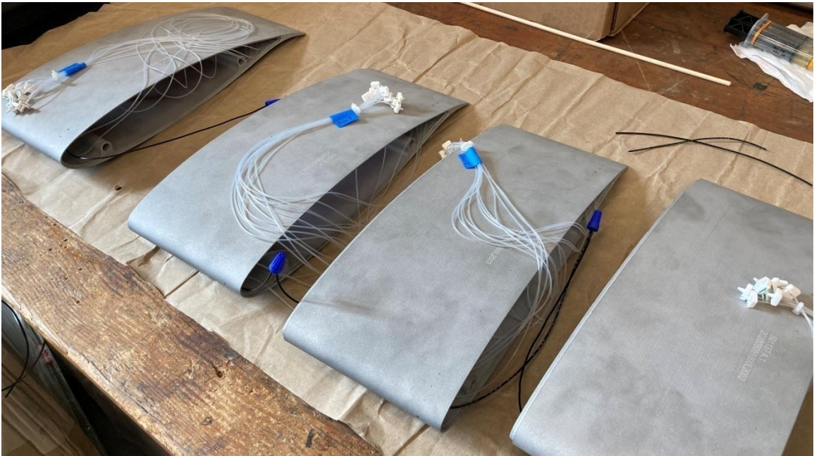
Figure 68: The Arrangement of Pressure Tubing, Adapters and Heating Pad Wires Before Bonding the Aluminum Print Sections into the Unified Center Section.
