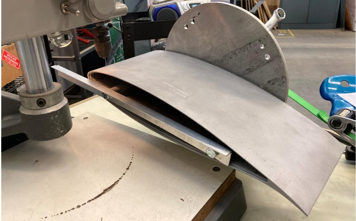
Figure 56: The Rotating Assembly Jig Used to Drill Pressure Tap Holes Normal to the Part Surface.
