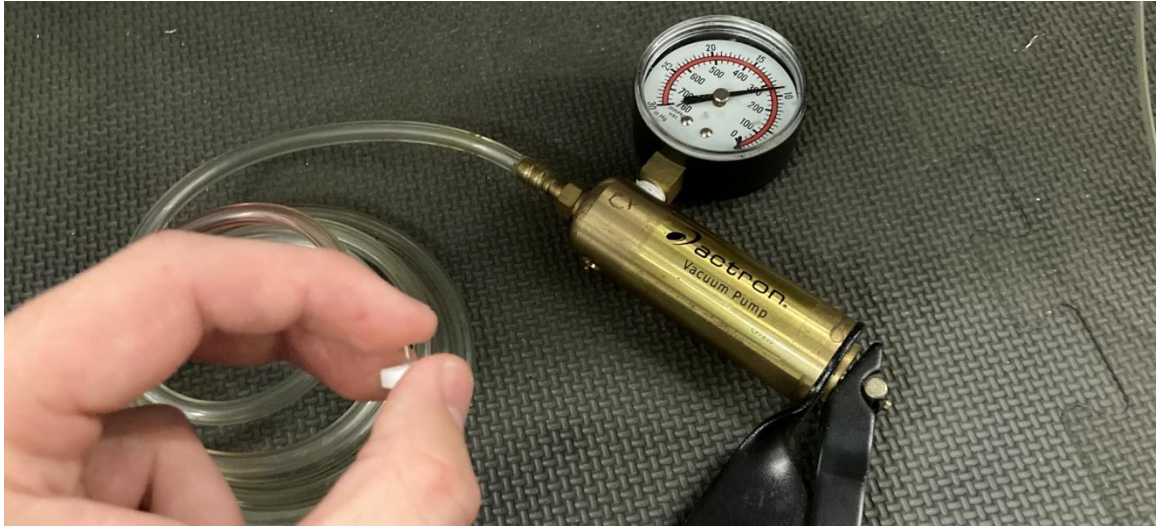
Figure 64: Checking a Pressure Line Adapter for Leakage Using a Hand-Held Vacuum Pump.
