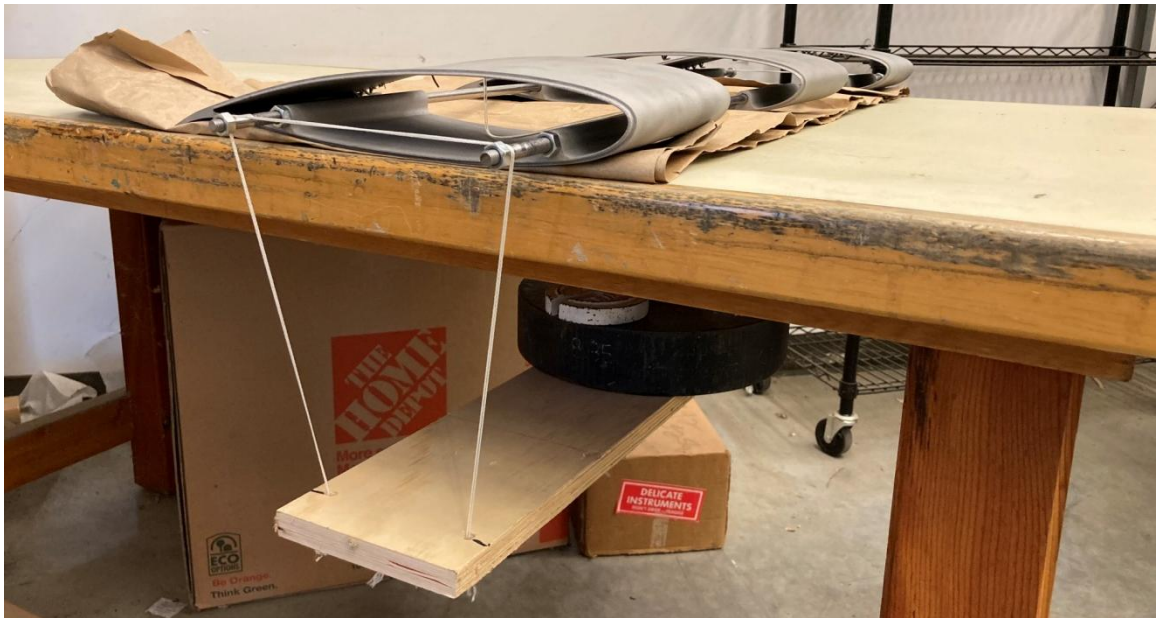
Figure 54: The Setup Used to Staticly Load the Wing Model's Structural Support Rods.
