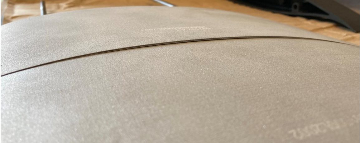
Figure 49: Profile Mismatch between End Profiles of the Raw Aluminum Printed Parts.
