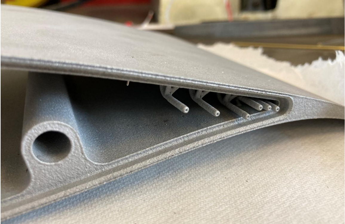
Figure 55: The Static Pressure Tap Barbs Printed Into the Structure of the Aluminum Center Section Parts.
