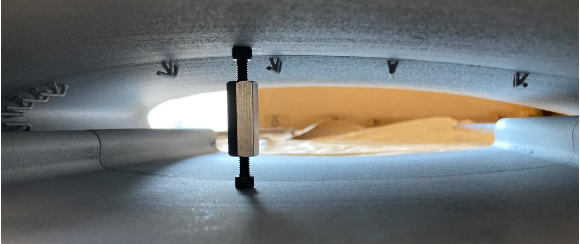
Figure 50: The Turnbuckle Mechanism Used to Forcefully Expand the Aluminum Parts and Remove the Discontinuity Created When Joining Them Together.
