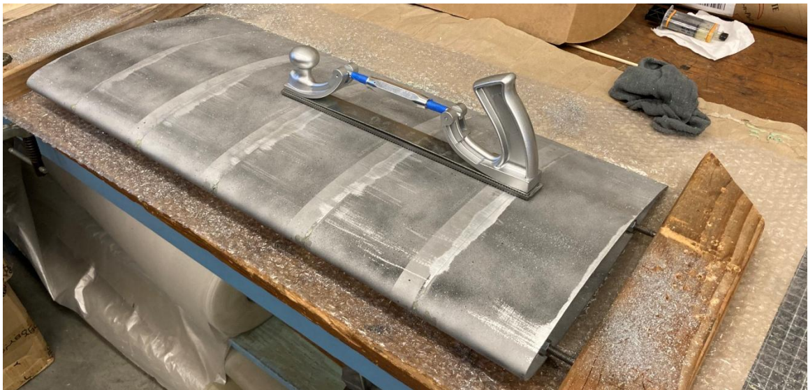
Figure 69: The Vixen File Visible with the Aluminum Center Section at the Early Stages of the Coarse Material Removal Process.
