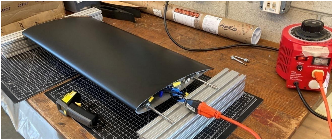
Figure 67: Image of the Revised Wiring Arrangement Being Connected Through the 3-Prong Plug and Tested for Maximum Attainable Steady-State Heat Capacity.
