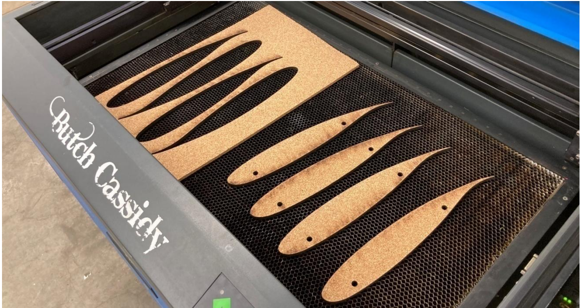
Figure 73: Image of the Cork Insulators After Being Produced by the Laser Cutting Machine.
