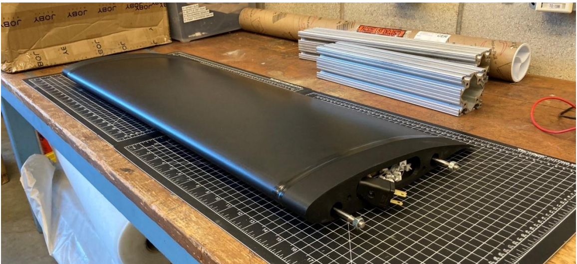
Figure 72: The Wing Model With the Vinyl Coating Applied and All Accessory Parts Installed.
