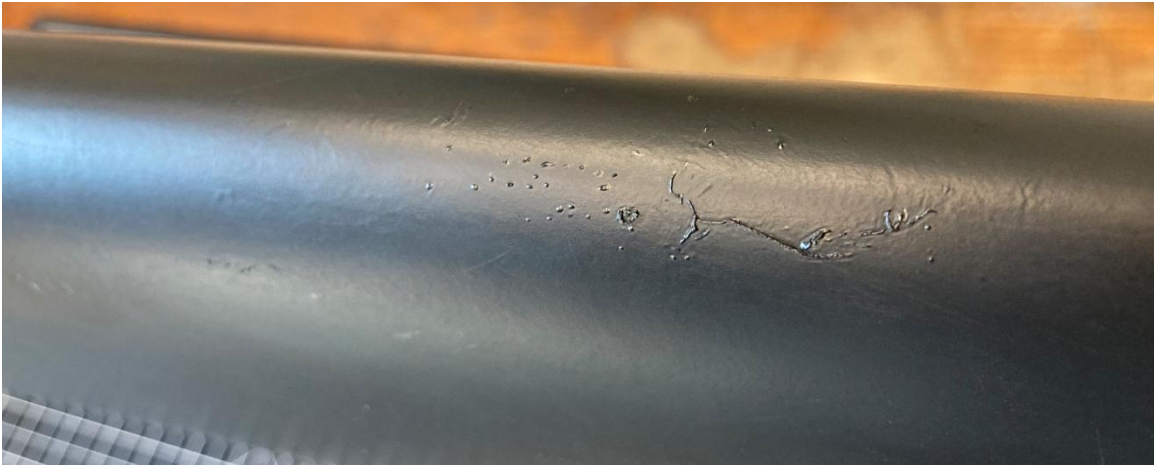
Figure 71: The Crease in the Second Vinyl Layer That Formed on the Leading Edge of the Model.
