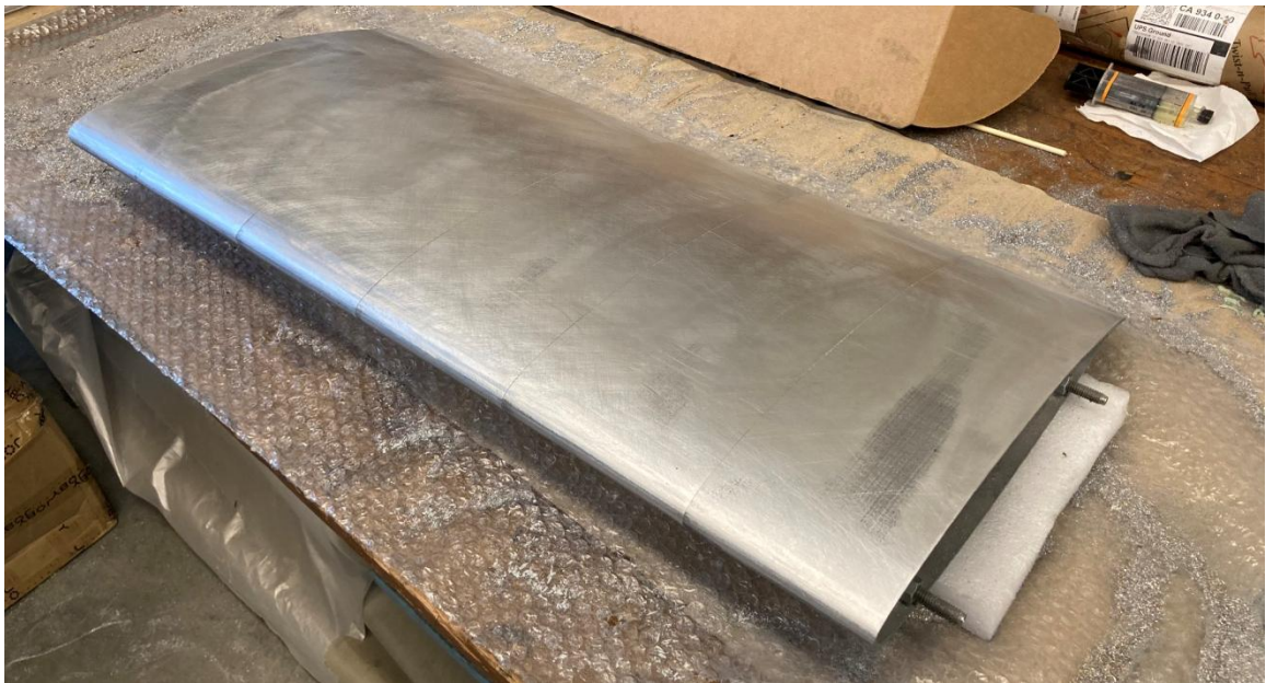
Figure 70: The Final Exterior Quality of the Aluminum Center Section after Filing and Sanding.
