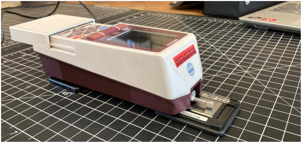
Figure 86: The Mitutoyo SJ-210 Surface Roughness Sensor Seen During its Calibration Procedure Using the Precision Sample Provided Alongside It.
