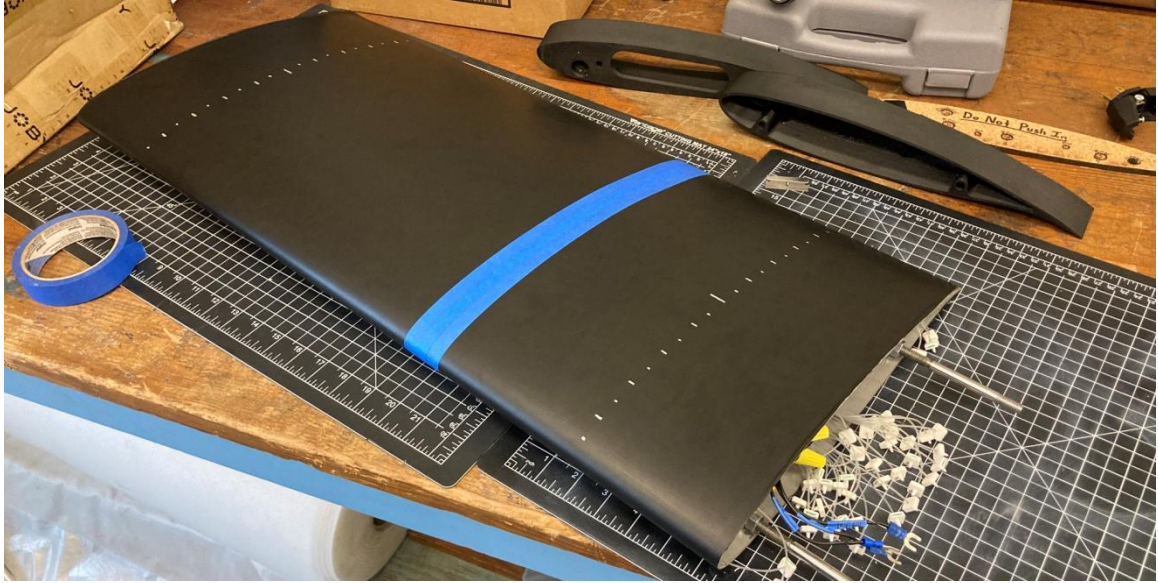
Figure 77: The Tape Marking Which Identified Where the Vinyl Coating Was Cut to Expose the Static Taps.
