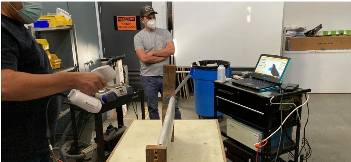
Figure 83: Image Taken During the Process of Scanning the Aluminum Center Section Using the Hand-Held Sensor Provided Alongside the Rendering Software.
