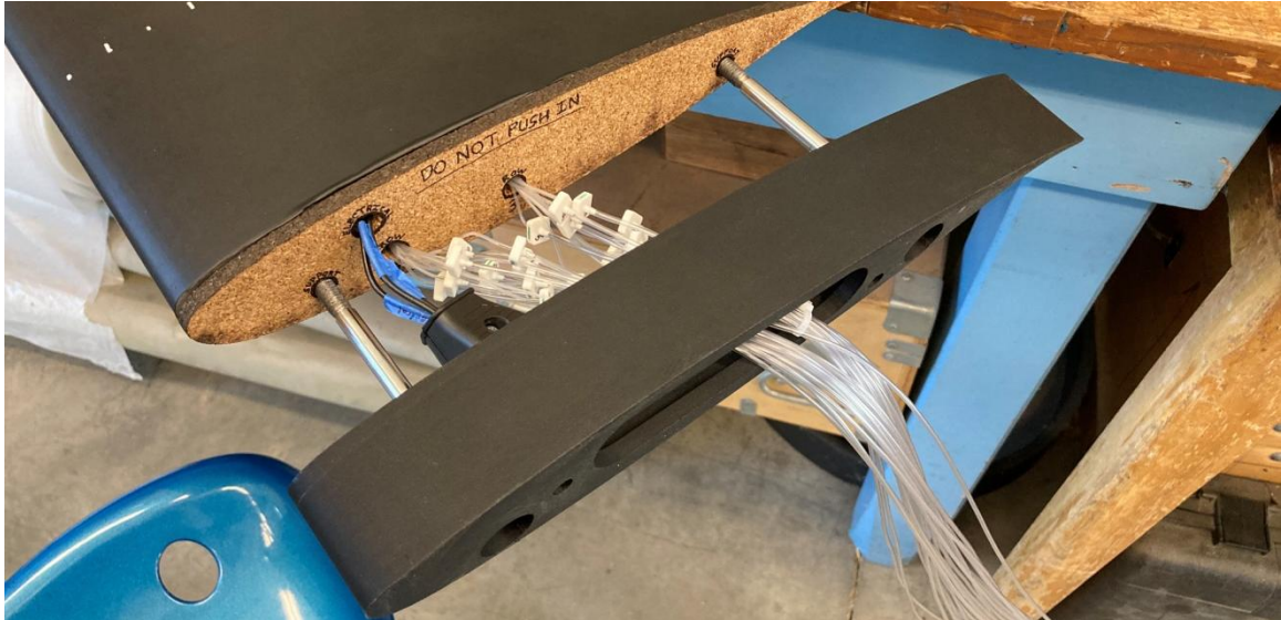
Figure 74: Organization of the Electrical Wiring and Pressure Tubing Through the Perforations in the Cork.
