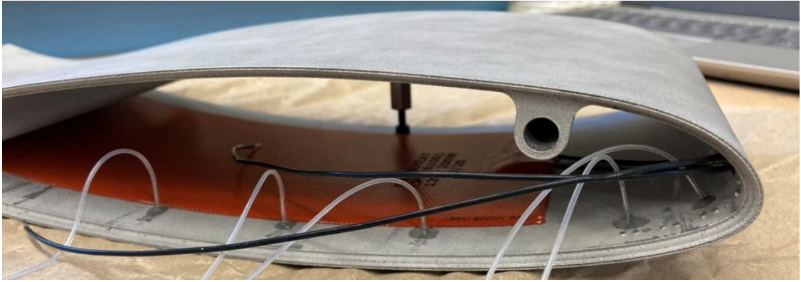
Figure 65: The Placement of the Internal Heating Element within an Individual Aluminum Print Part.
