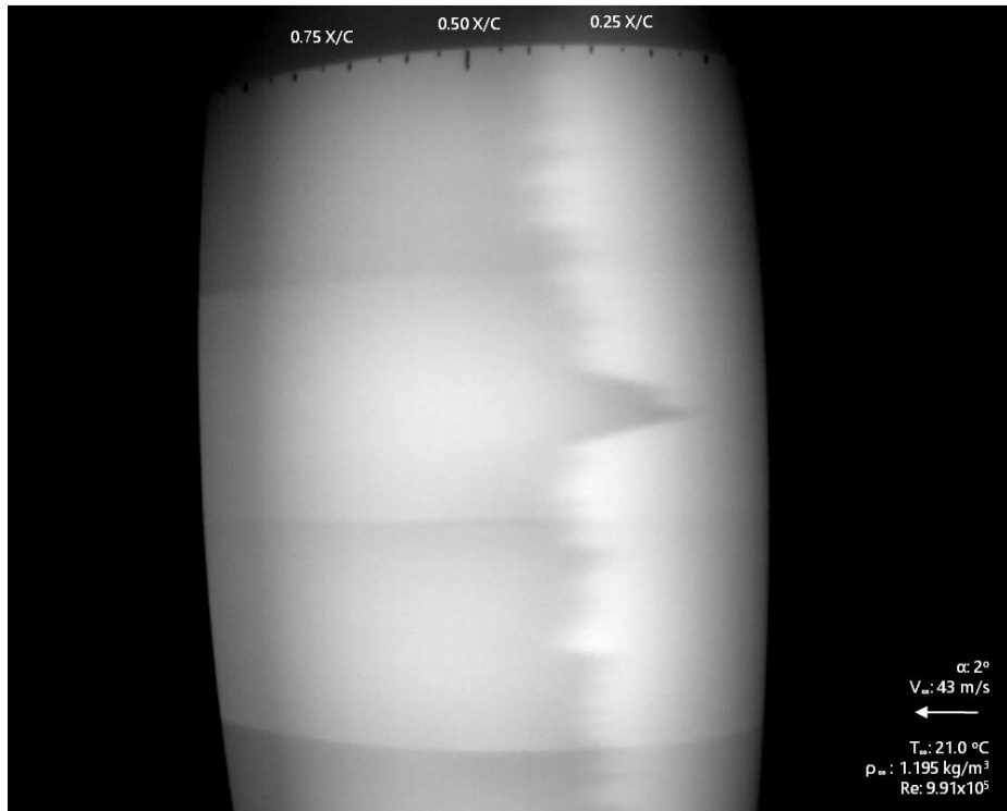
Figure 98: Infrared Thermographic Image of the Wing Model at an Effective Aerodynamic Pitch Angle of 2^\circ .
