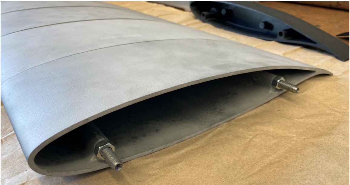
Figure 52: Testing the Fit and Length of the Primary Steel Support Rods.
