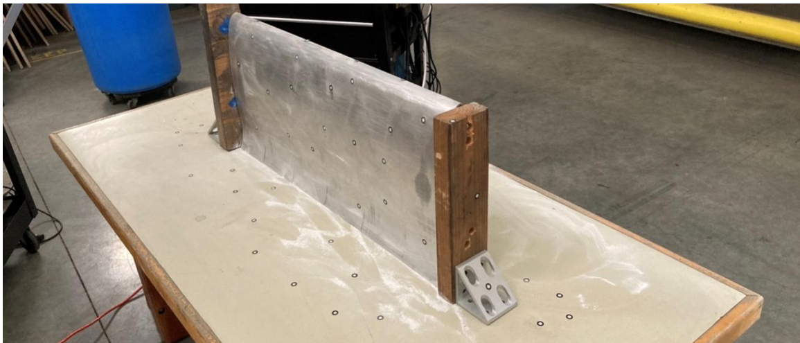
Figure 82: The Setup Used to Take 3D Scan Measurements of the Aluminum Center Section.
