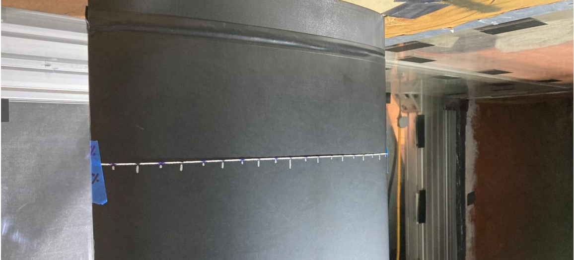
Figure 90: The Measurement Method Used to Mark the 0.05 x/c Indicators on the Model Surface.
