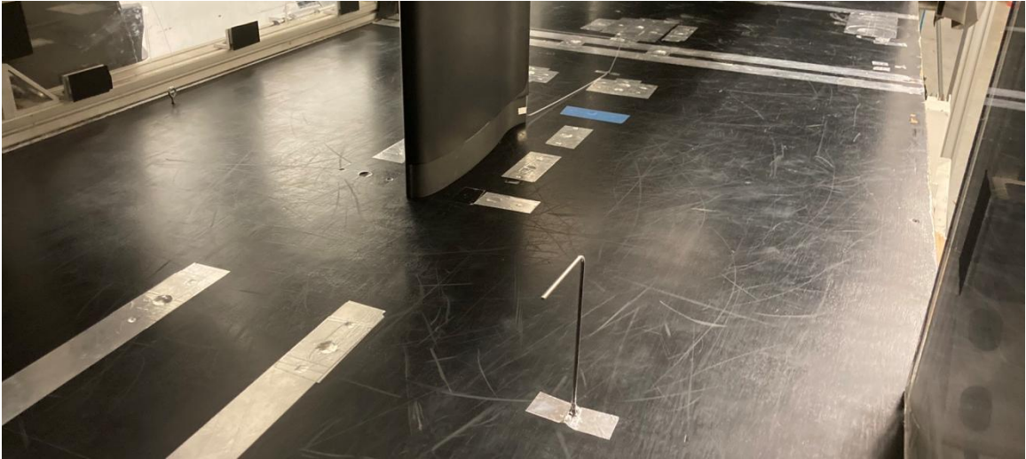
Figure 94: View of the Pitot-Static Probe Installed in the Test Section Floor Near the Wing Model.
