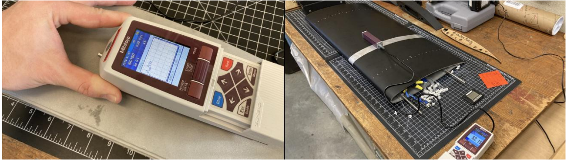
Figure 87: Use of the Surface Roughness Meter to Measure the Raw Printed Aluminum (Left) and the Vinyl Covered Aluminum (Right) of the Wing Model Center Section Parts.
