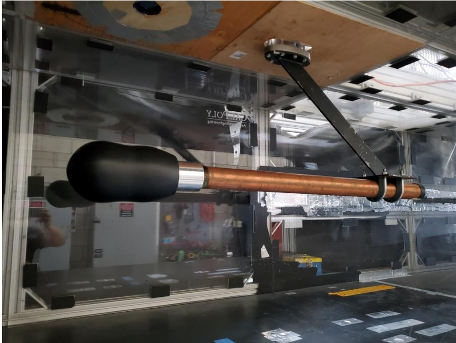
Figure 22: The Validation Mounted in the Cal Poly LSWT Test Section Using the Same Mounting Arm as the Ducted Nacelle Model. The View Port for the Infrared Camera was Located Above the Model.
