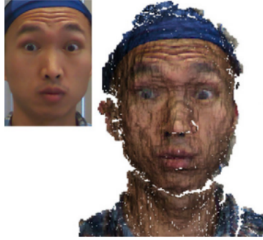
Figure 3.11: Example of raw depth-data generated by a RGB-D camera (right) with the same capture represented in RGB form (left) [20].
