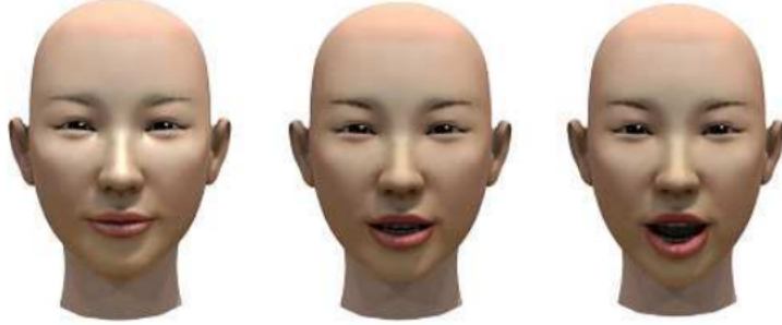
Figure 3.3: The resting blendshape pose (left) is combined with the mouth-open blendshape pose (right) to create the novel pose (middle). To animate the mouth opening, the weight of the mouth-opened blendshape would be increased over time [11].
