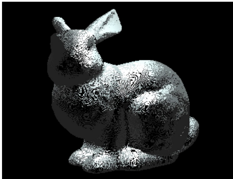
Figure 4.5: A render of a bunny that has its normals calculated with the immediate neighbor gradient approach. This output image shows a lot of noise and shading discontinuities, but it demonstrates the potential to approximate voxel normals from surrounding voxels.
