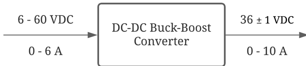
Figure 1: Level 0 Block Diagram of DC-DC Buck Boost Converter
