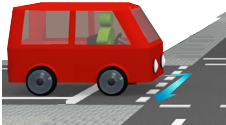
Figure 4.4: A recommendation on the visual aspect of the AV's external HMI based on study results
