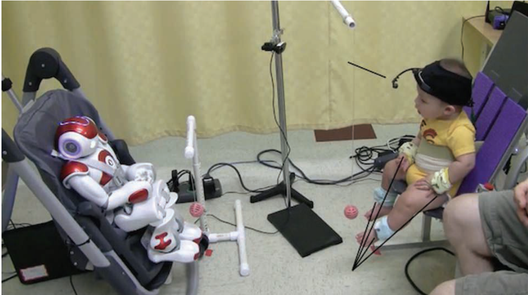
Figure 2.3: An experimental setup in which an infant interacts with an NAO robot while the labeled sensors (an eye tracker and inertial sensors) and additional sensors (RGB cameras and a Kinect One RGB-D sensor, which are not shown in the field of view of this image) capture information about the infant-robot interaction. Adapted from [21].
