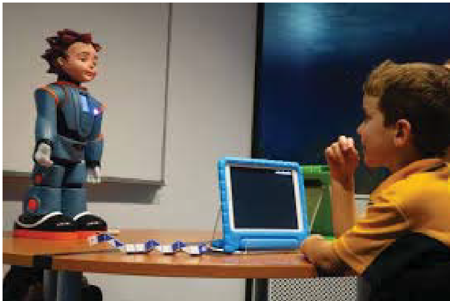
Figure 2.4: The humanoid robot, Milo, developed by RoboKind. It can walk, talk and model human facial expressions. It delivers lessons verbally to teach social behavior and emotional aspects. Adapted from [22].
