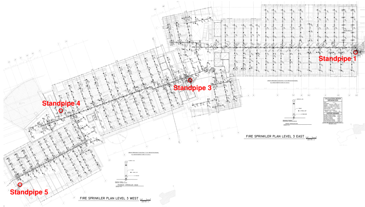
Figure 21. Building layout with standpipes.
