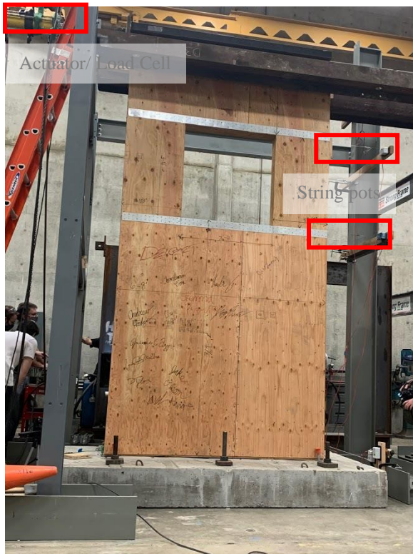
(a) Instrumentation on Front of Wall
