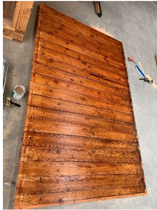
Figure 7- Third Coat Applied to Left-Hand Panel
