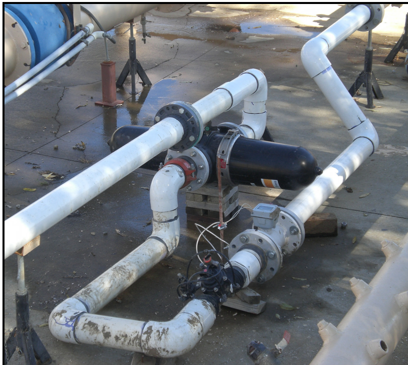
Figure 4. Test configuration for 4-inch magnetic meter
