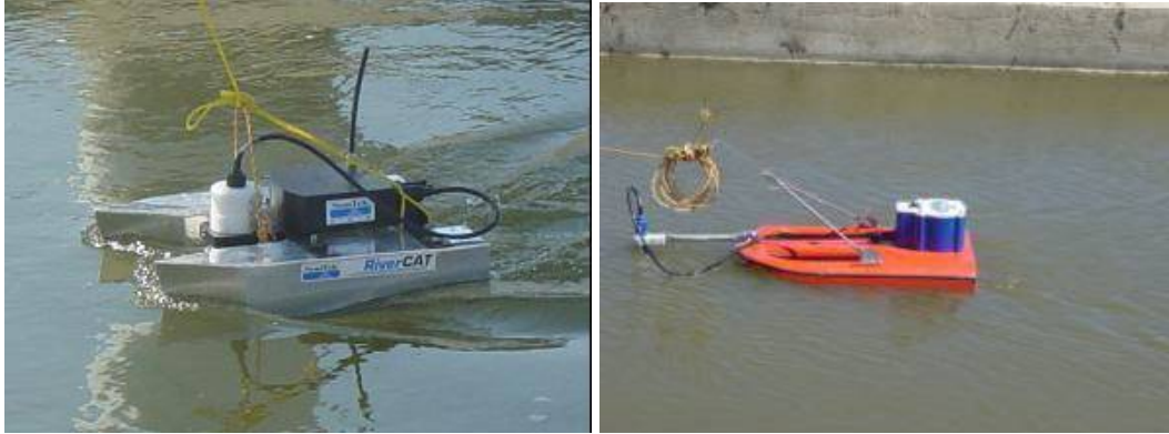
Figure 1. Boat-mounted Acoustic Doppler Profilers collecting flow rate and cross-sectional measurements in irrigation canals
