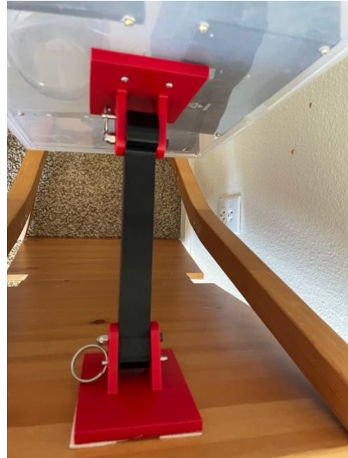
Mount appearance with screws and pins properly located in the mount
