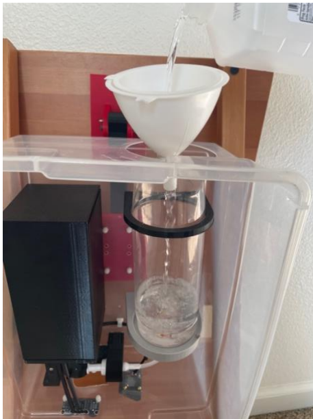
Step 5: Unscrew the cap of the reservoir and fill using sanitizer, screw cap back on when reservoir is at desired level
