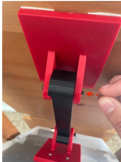
Step 3b: Screw on the nut to the protruding threads of the screw
