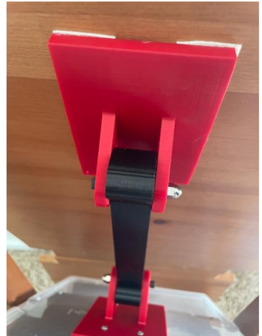
Mount appearance when screw is properly located in the mount
