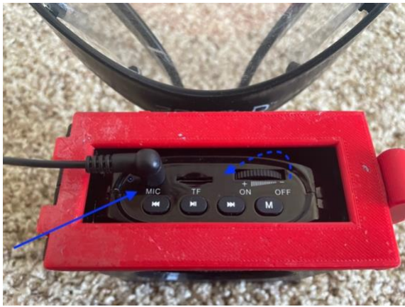
Step 3: Spin the wheel towards "ON" to increase the volume, plug in the microphone into the audio jack
