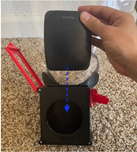
Step 1: Insert the speaker into the case
