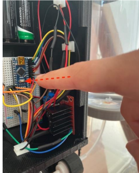
Step 8: Press reset button on Arduino Nano to calibrate, system is now ready to operate
