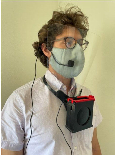
Step 4: Put on the face shield with the support resting on your collar bones, adjust angle for comfort; rest microphone over ears or neck
