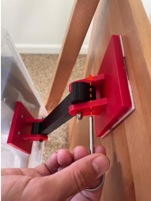
Step 4: Line up the pin with the pin hole for your desired position
