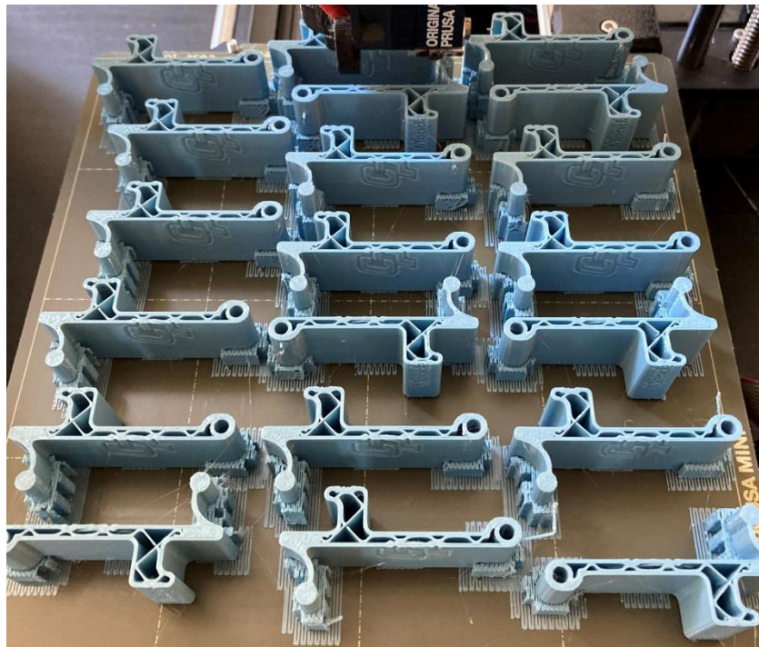
Figure 38: Pill box lids being 3D printed.
