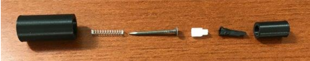
Figure 27: 3D printed locking, click-pen mechanism, disassembled.
