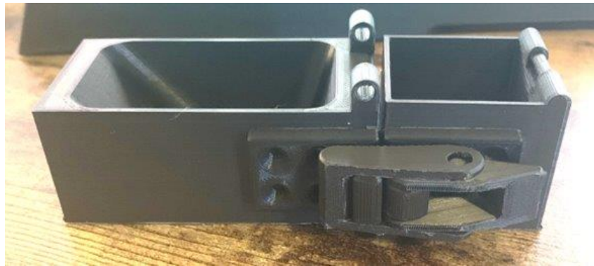
Figure 25: 3D printed toggle latch, attached to pill containers.
