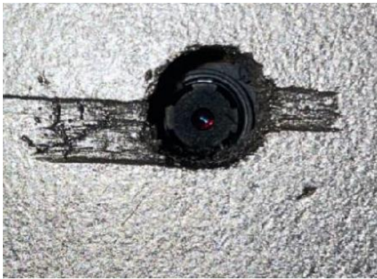
Figure 43: Camera Cutout Exterior
