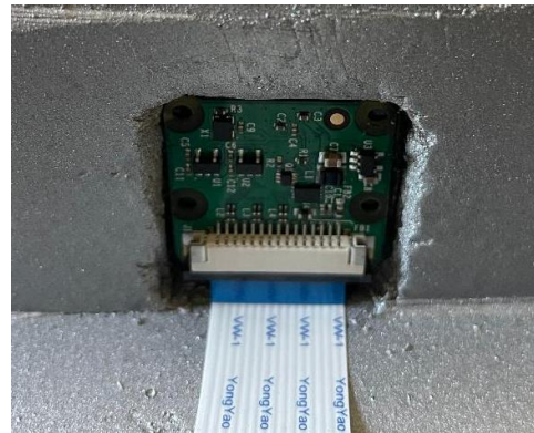
Figure 44: Camera Cutout Interior
