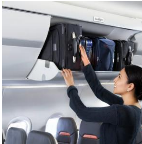
Figure 6. The phenolic resin glass fiber reinforced prepreg is used in the manufacturing of the overhead cabins of an A220 aircraft. [11]
