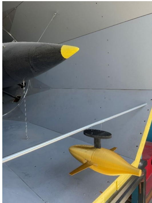
Figure 58: UAV model suspended behind outlet of wind tunnel during test.
