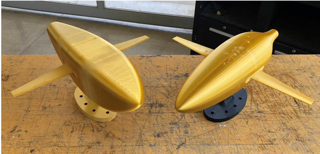
Figure 57. Complete 3D-printed prototypes of UAV models with symmetrical airfoil fuselage (left) and axisymmetric fuselage (right). Both models are approximately 18 inches long, 16 inches wide, and 9 inches tall.
