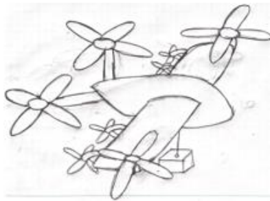
Figure 8. Quadrotor Configuration with Wings and Pusher Propellers
