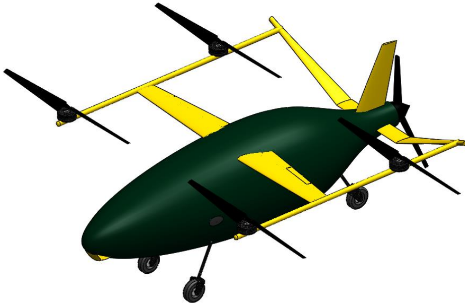
Figure 44. Final UAV design featuring propeller at the back and new fuselage shape designed to minimize drag.
