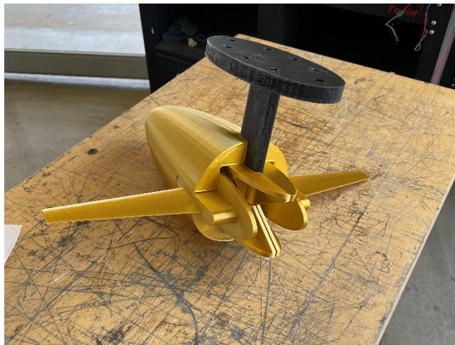
Figure 56. Front half of one of the scaled-down UAV models with stand, retainers, and wings installed in the internal cavity. The wings and stand are located using slots in the fuselage.
