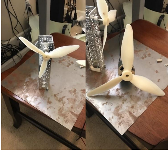
Figure 60. Input assemblies for wind turbine structural prototype
