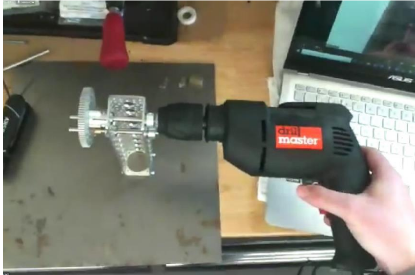
Figure 50. Hand drill test of exploration activity prototype
