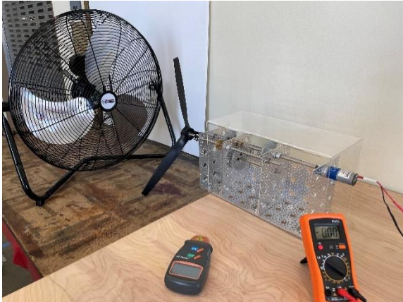
Figure 68. Wind turbine and torque increaser geartrain test
