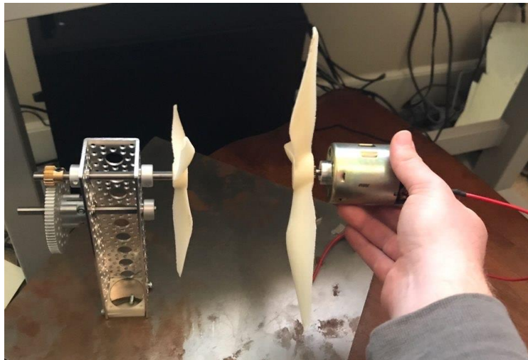
Figure 61. Testing of wind turbine structural prototype
