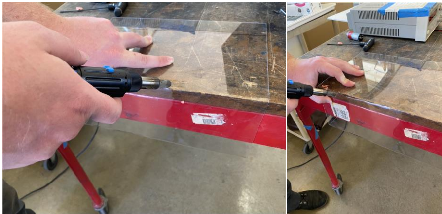
Figure 71. Bending acrylic for turbine housing using butane torch
