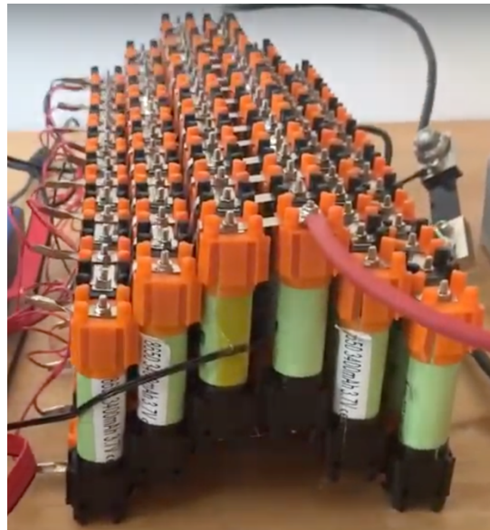
FIGURE VI TOP VIEW AND SIDE VIEW OF THE 16S X 6P BATTERY PACK.
