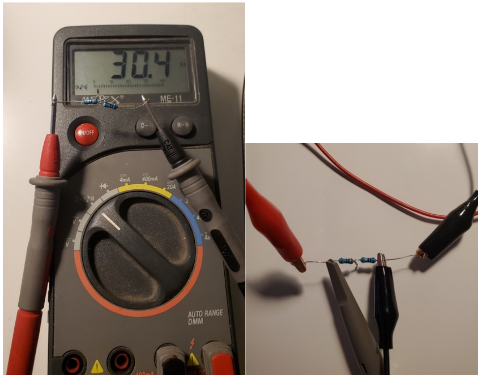
FIGURE 38: MEASUREMENT AND SETUP OF HEADPHONE “DUMMY LOAD”
