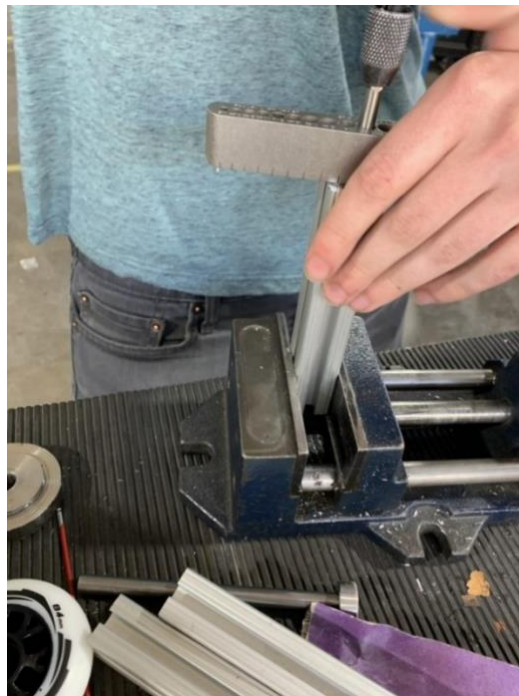
Figure 34: Tapping the end profile hole of a 6" T-slot.
