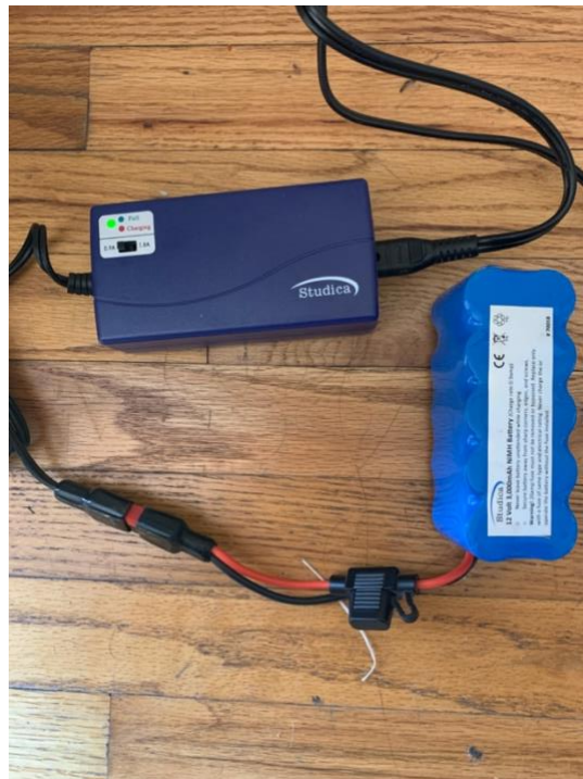
Proper Terminal Connections
