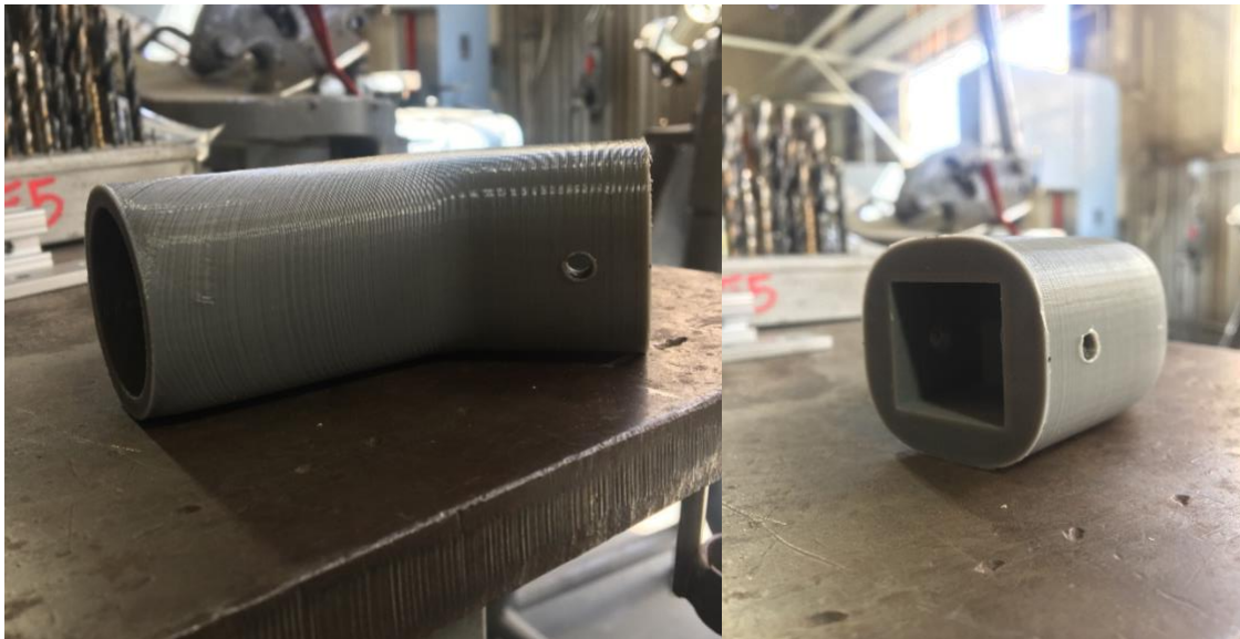
Figure 33: 3-D printed PVC pipe connector
