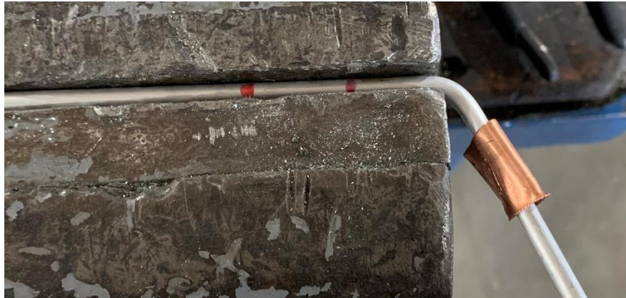
Figure 32. Bending of the flexure probe tip
