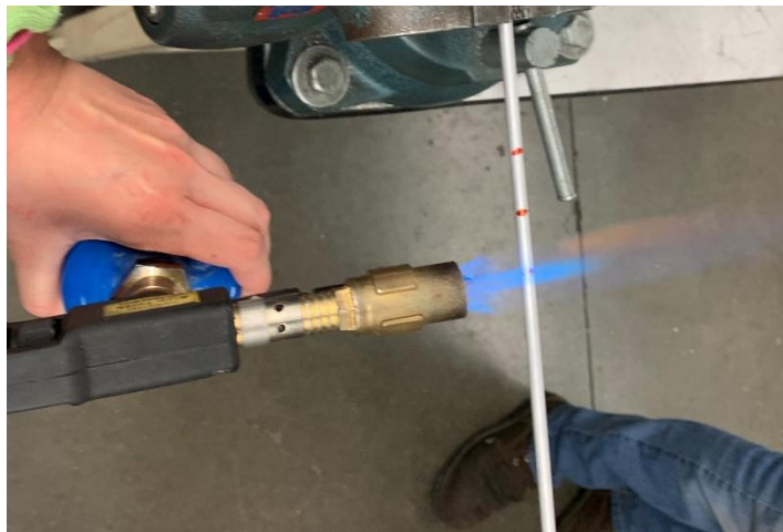
Figure 28. Heating of flexure rod for bending to demonstrate color change of flame.
