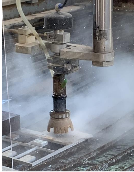
Figure 27. Tool base plate in the process of being waterjet cut.
