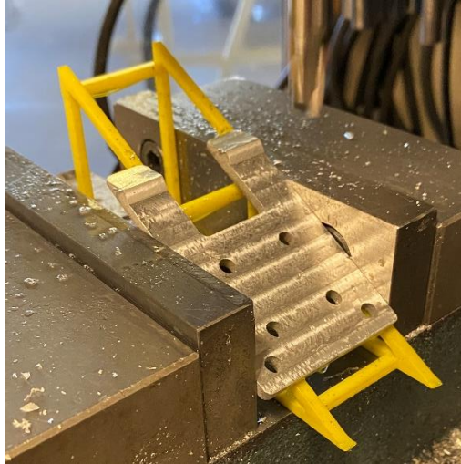
Figure 31. Mill set up for milling angled surfaces of tool base plate.
