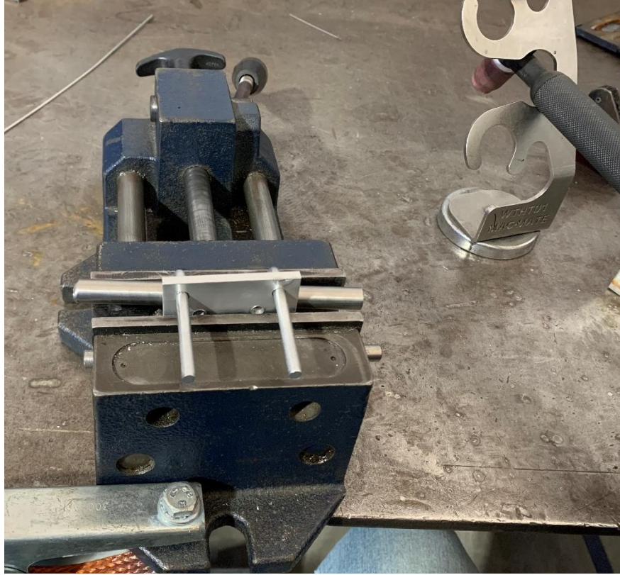
Figure 34. Weld setup of tool component before welding has been completed
