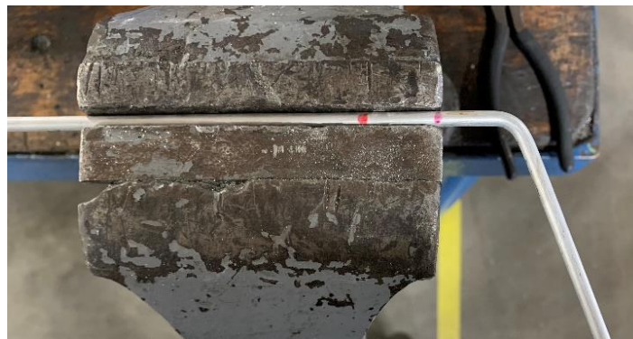
Figure 33. Resulting probe bend after steps 2-7
