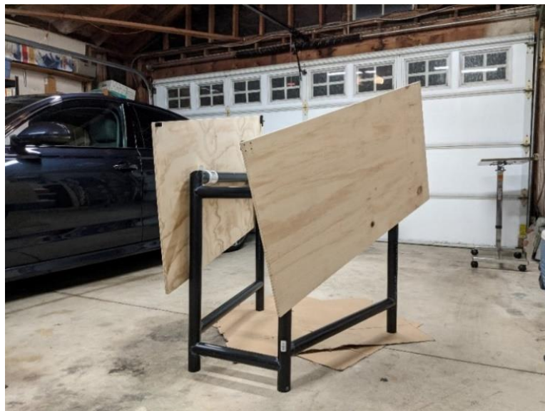
Figure 35: Concept prototype built from ABS piping and plywood.
