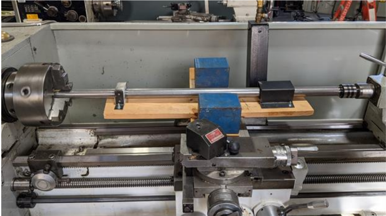
Figure K4: Life testing setup in a lathe.
