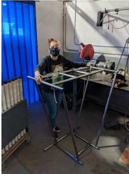
Figure Q 1: The welding jig closes the open part of the trapezoid base.
