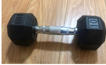
Figure I7: 10 lb. weight to be dropped to create an impact load.
