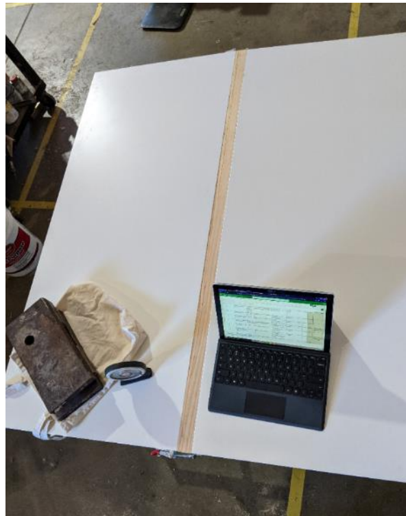
Figure 65: Loads being applied at the testing point on the table.
