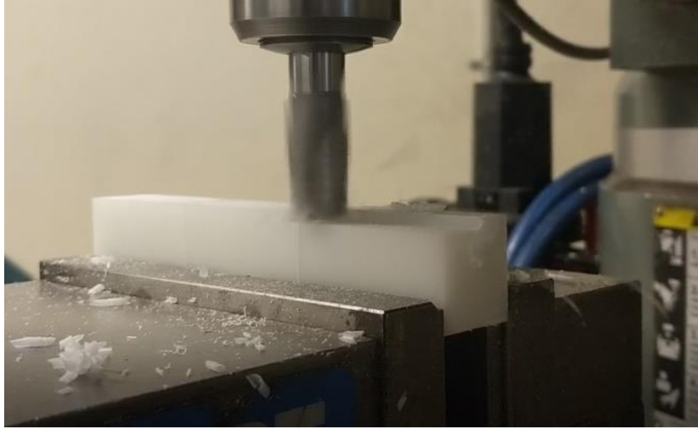
Figure 51: UHMWPE bushing milling process.
