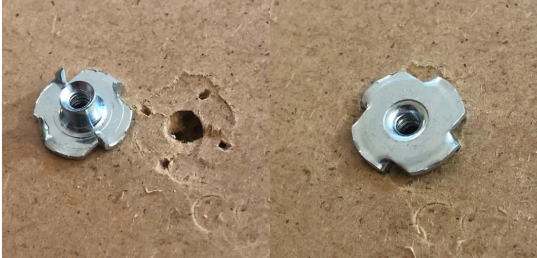
Figure I10: Everbilt zinc tee nut installation failure.
