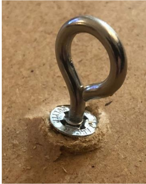
Figure I12: EZ Anchor installed with adhesive destructive test.
