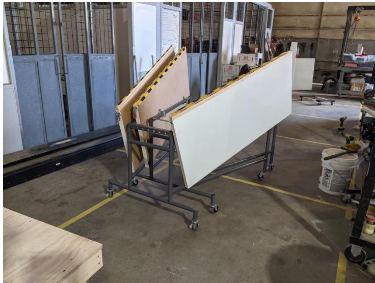
Figure 49: Installed warning label across tongue/groove feature.
