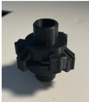
Figure 17: 3D-printed bayonet locking mechanism with both halves locked together.
