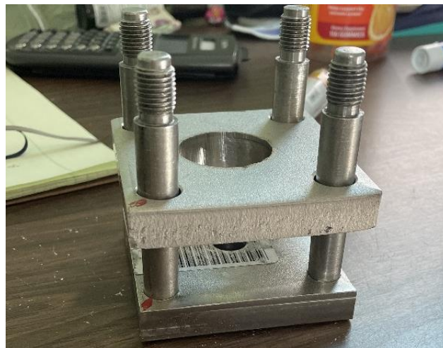
Figure 25: The top and bottom plate with pins press fitted. Does not include the bayonet connector, jounce bumper, or nuts.
