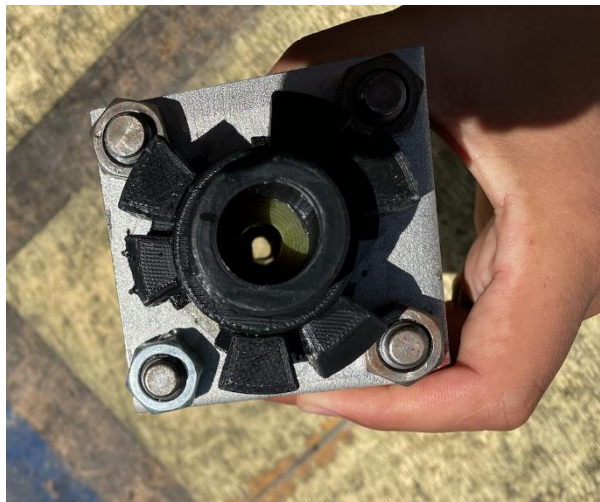
Figure 38: Checking to see if the epoxy seal between the bushing and bayonet locking mechanism succeeded in keeping the inside of the bayonet locking mechanism dry.
