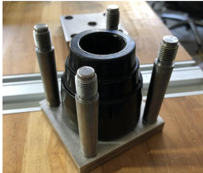
Figure 26: The bottom plate with jounce bumper set in place
