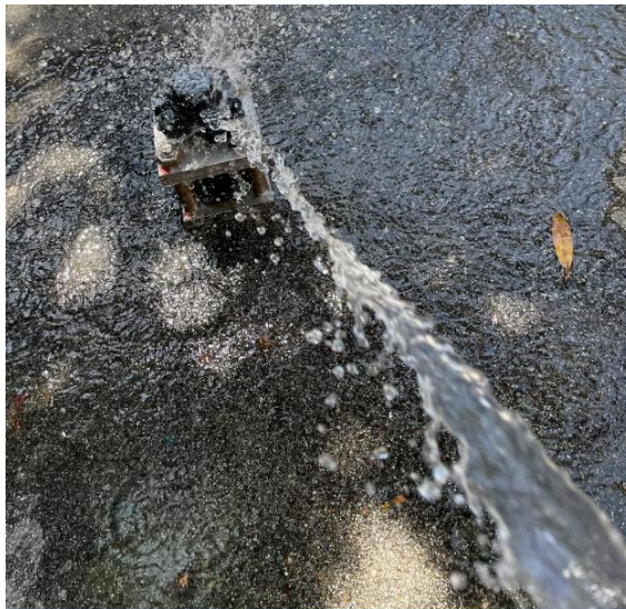
Figure 36: Watertight test of epoxy seals between the bushing and bayonet locking mechanism.
