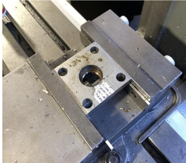
Figure 24: The top plate held in the mill vise.
