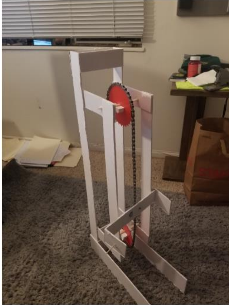
Figure 11. An image of a prototype built for the “Conveyor Belt” design. In this design, the carriage is pulled directly by the rotating chain. Once the carriage reaches the top of the chain, it is forced to rotate over the top gear.
