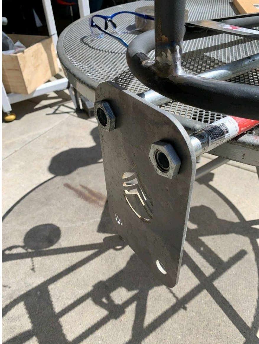
Figure 28. The arm clamp plate affixed to the 24" threaded pipes with pipe nuts. As shown in the image, Mr. Jauregui's Army insignia was cut out of the arm clamp plate in order to remove material and to pay homage to his service.
