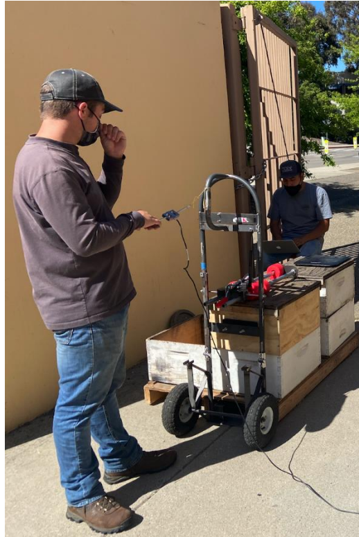
Figure 34. Here Ryan and Jose perform the weighted bee box pull procedure. This test was performed using weight ranging from 40-80 lbs. to ensure the clamping arm would apply sufficient force on the bee box.
