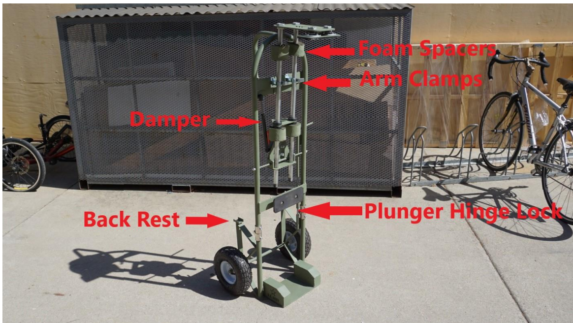
Figure 26. A picture of the final Beekeeper Assist, with changes made during the manufacturing process labelled in red; more specific details about these changes can be found in Appendices K through N.
