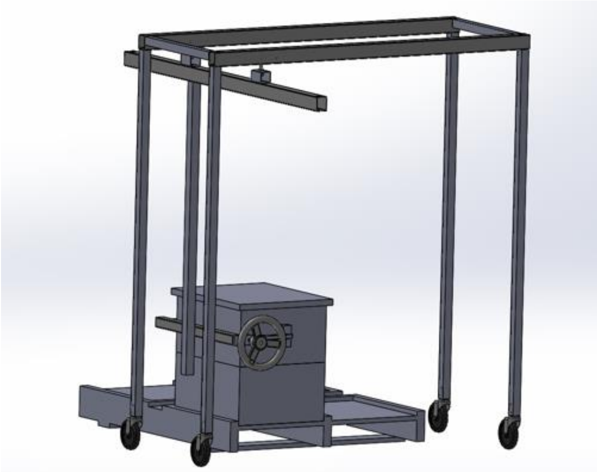
Figure 12. An isometric view of the “Moving Crane” design built in SolidWorks. In this design, the box is gripped by a wheel-tightened clamp attached to the crane above. A winch would be activated.
