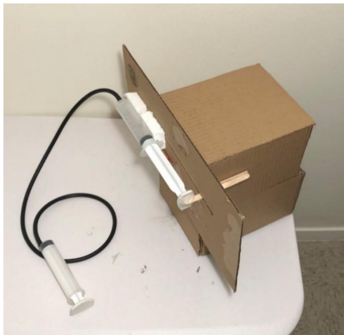
Figure 9. A picture of an “attach to box” prototype our group built. This prototype was meant to represent how a hydraulic/pneumatic system could be used to clamp holding plates to the box.
