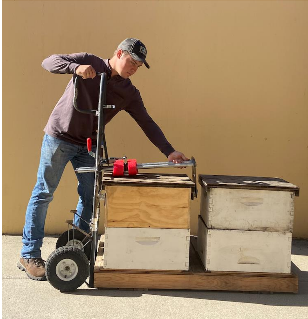
Figure 36. The test that determined how long it would take to set-up the Beekeeper Assist which is relatively the same about of time it would take Mr. Jauregui to lift and rotate the bee box out of the way for him to inspect his beehives.
