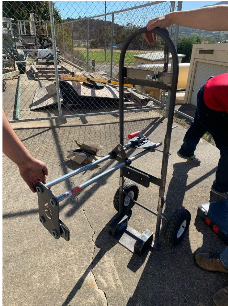
Figure 32. The fully assembled verification prototype in the down position. This image does not include the back support, the spacer, or the rotation blocker, but everything else is in completion.
