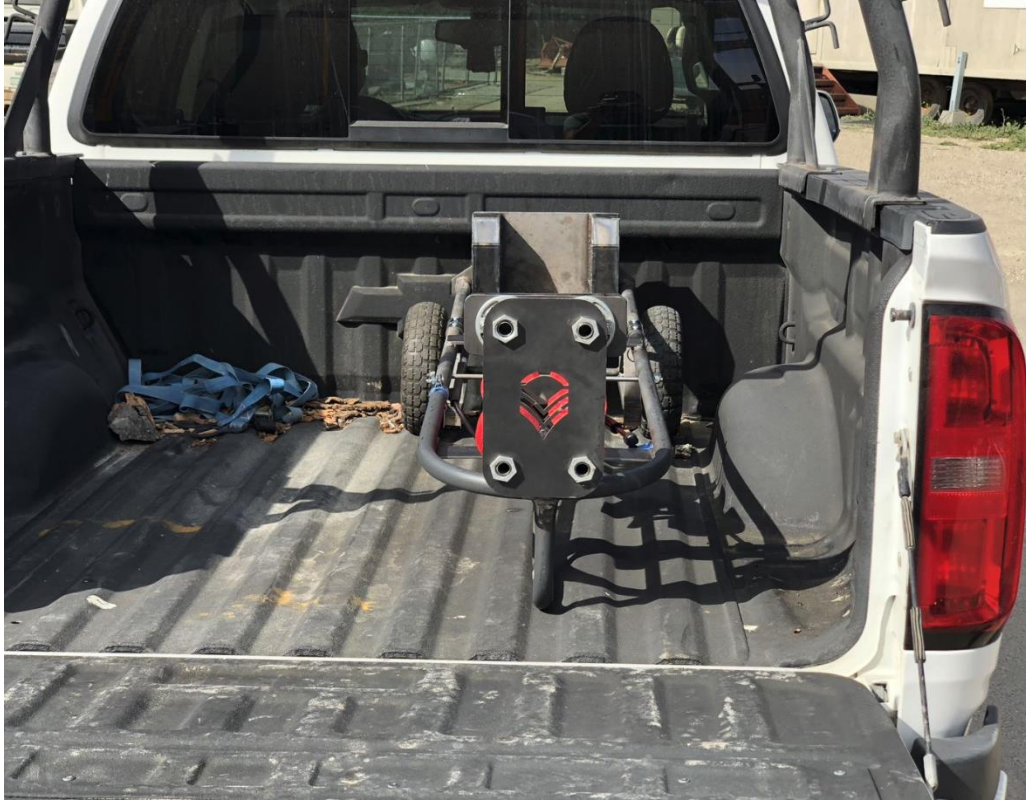
Figure 35. The test ensuring that the Beekeeper Assist will fit comfortably in the bed of Mr. Jauregui's pickup truck. While we did not measure the dimensions of this truck bed, we know that the truck bed in this image is smaller than Mr. Jauregui's truck bed.
