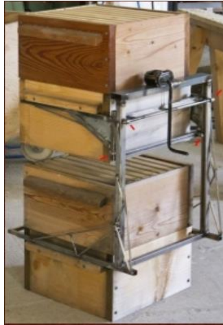
Figure 5. A bee box lifting device built by Kai Serschmann.
