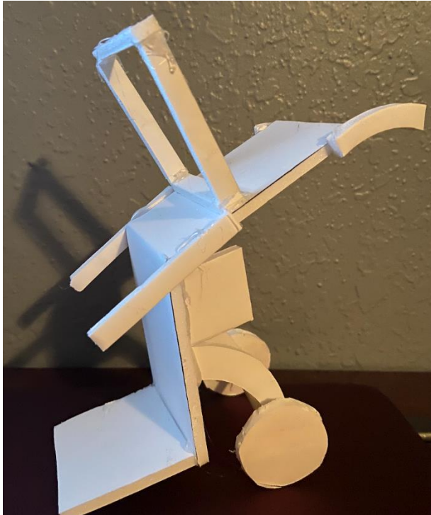
Figure 3. A picture of another multi-purpose, first-generation prototype. This prototype is mainly meant to emulate rotation through the use of hinge. The user would pull down the top portion of the dolly to rotate the box back. The whole thing is attached to a dolly mechanism.
