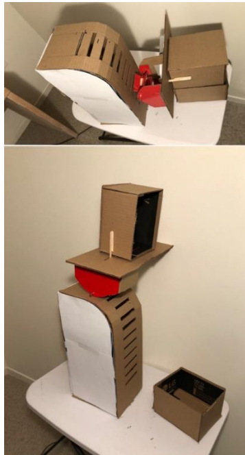
Figure 1. A picture of a multi-purpose, first-generation prototype. This prototype was meant to emulate horizontal movement, vertical movement, and rotation through the use of a rack and pinion (the carriage has a “gear” and “motor”). It also depicts the “attach to box” sub-function through the use of a syringe clamp mechanism.
