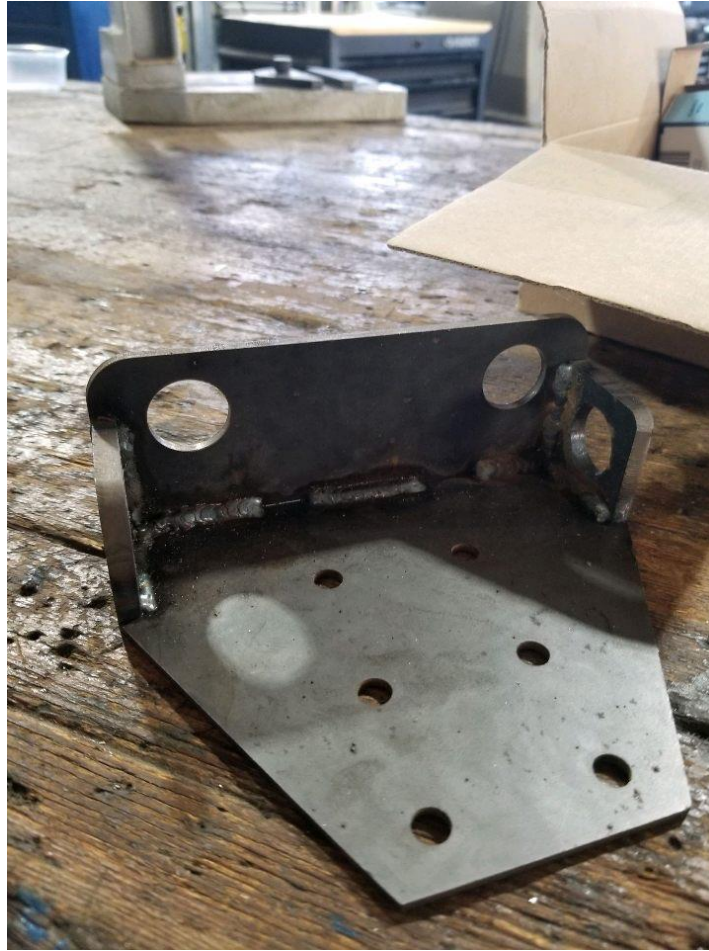
Figure 30. The welded hinge piece.
