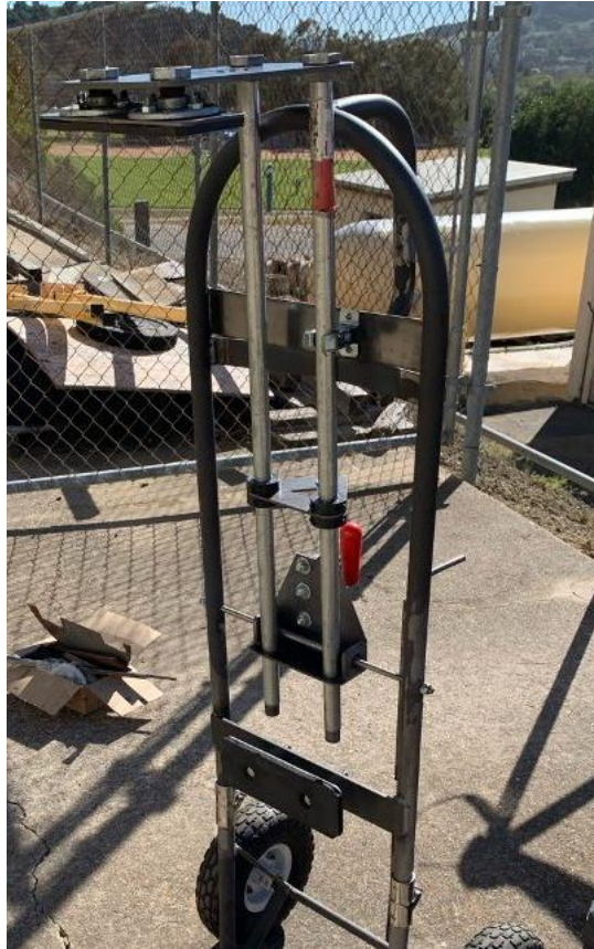
Figure 27. Upper dolly frame with the back support plate, cross bar, dowel for locking mechanism, and clamp for the arm on when it is in its upright position, as shown above.
