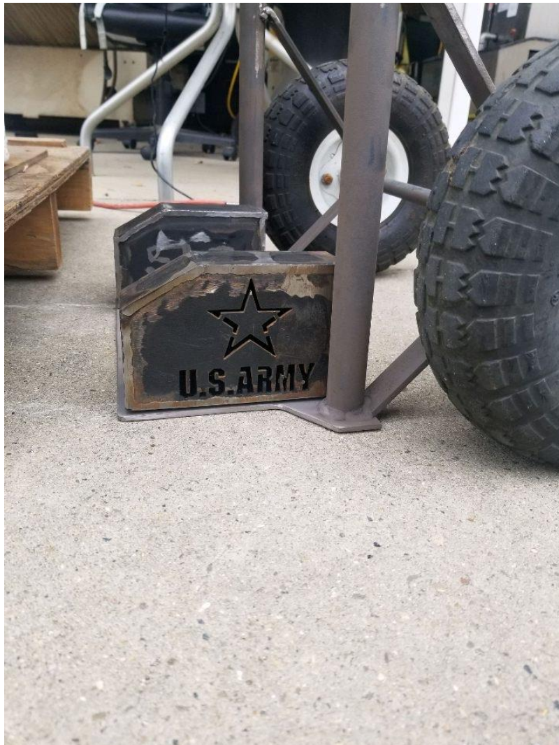
Figure 31. The final version of the dolly's forks. In this image, the forks have been welded to the base plate but have not yet been powder coated. This image also shows the U.S. Army logo we had cut into the forks to pay homage to Mr. Jauregui's service.
