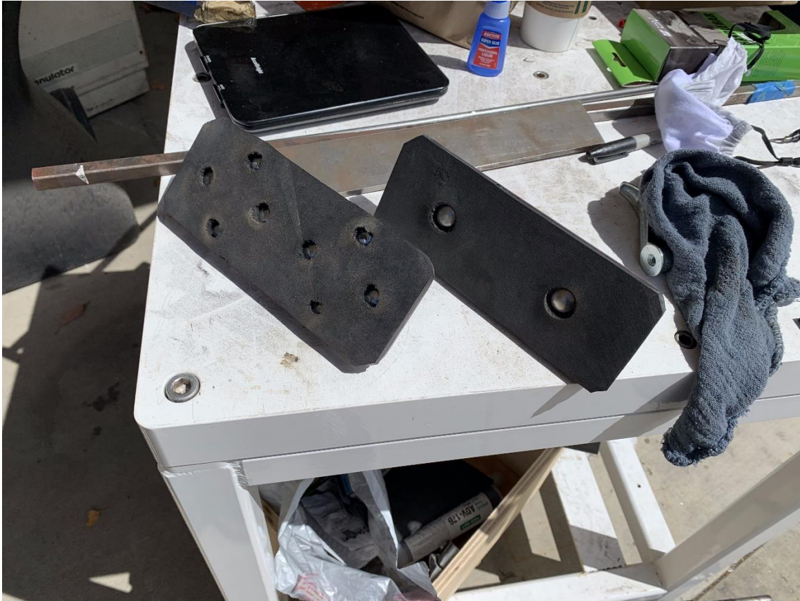
Figure 29. The rubber friction pads adhered to the front and back box plates, respectively from left to right.
