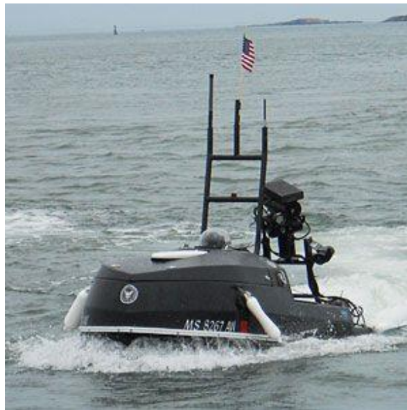
Figure 2.1. US Navy’s prototype for Blackfish, a harbor defense device used to scout and potentially eliminate abnormalities in sonar scanning (Hambling).
