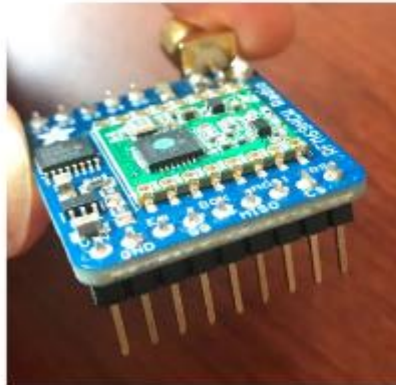
Figure 1. Pin connectors in RFM69HCW board.
