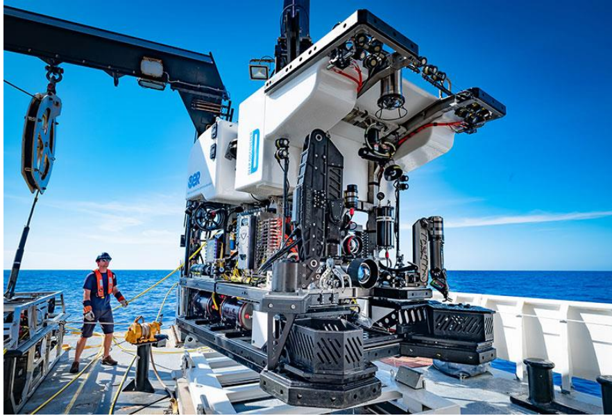
Figure 2.5. Deep Discover by the Global Foundation of Ocean Exploration, with caged propellers on the bottom of the device (US Department of Commerce).
