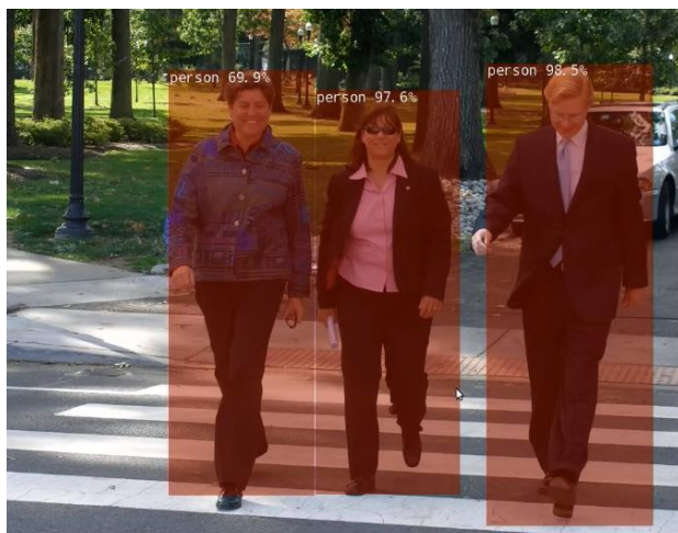
Figure 5.5. Image recognition done by the Jetson. Contains probability calculation results with each person.
