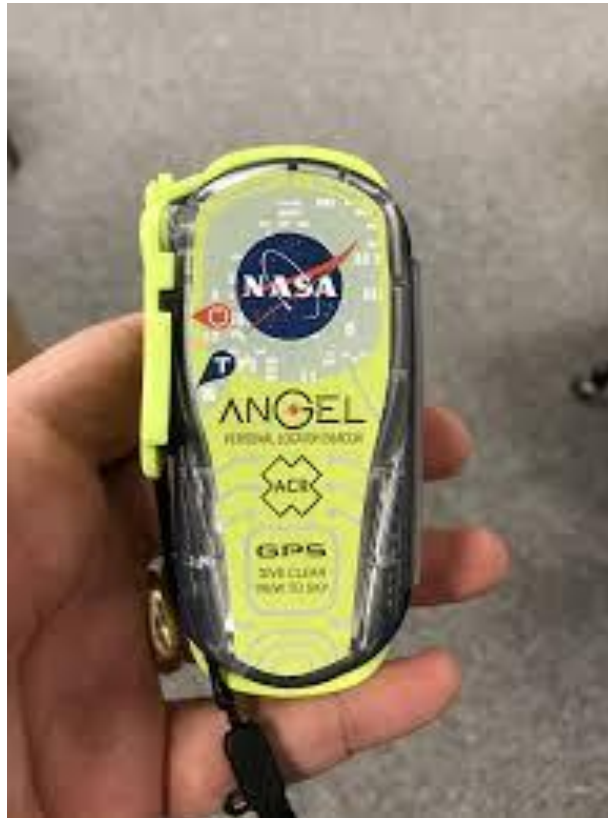
Figure 2.3. NASA’s personal locator beacon, ANGEL (Mazzuca).
