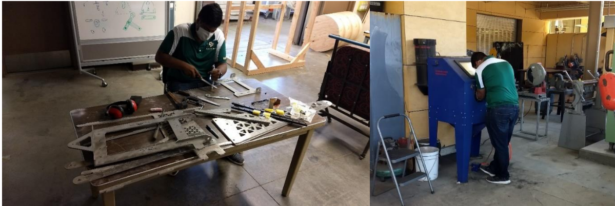
Figure 121. Deburring and filing the parts (Left) and cleaning them with a sandblaster (Right)
