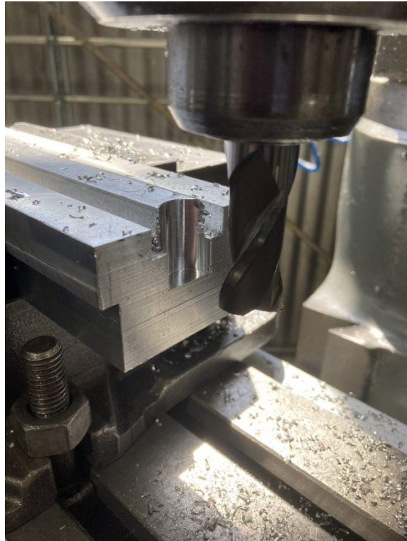
Figure 105. Milling the Double Pin Guide Slot on the Latch
