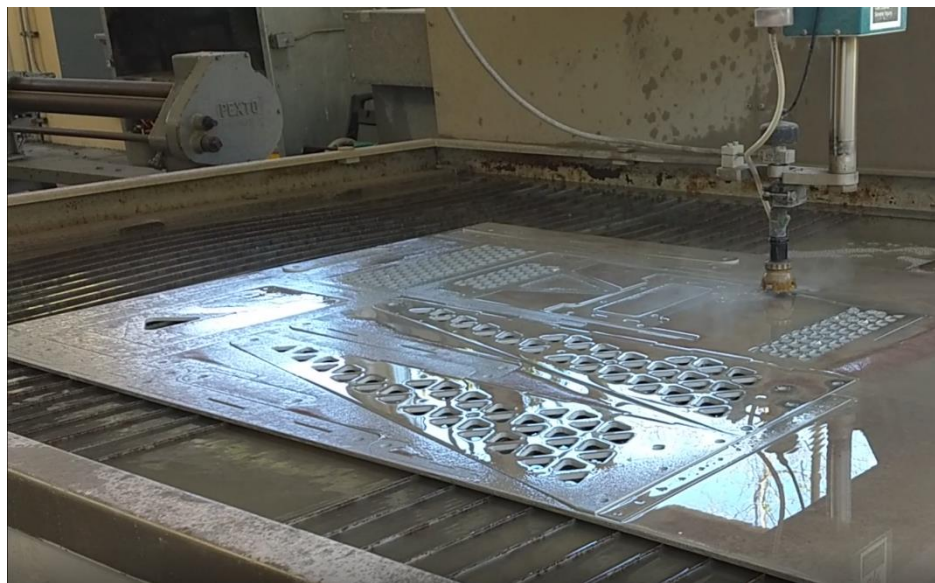
Figure 117. Final cut on the waterjet
