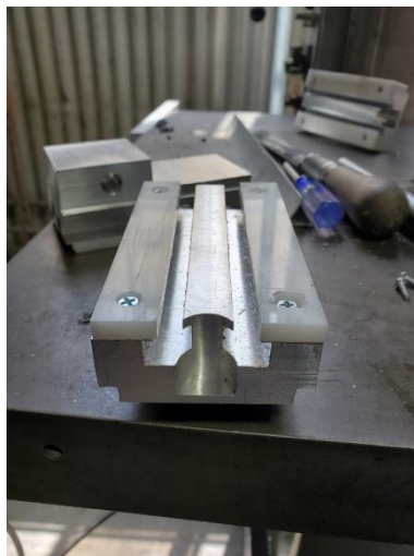
Figure 109. Completed Single Latch with Delrin Slides Attached
