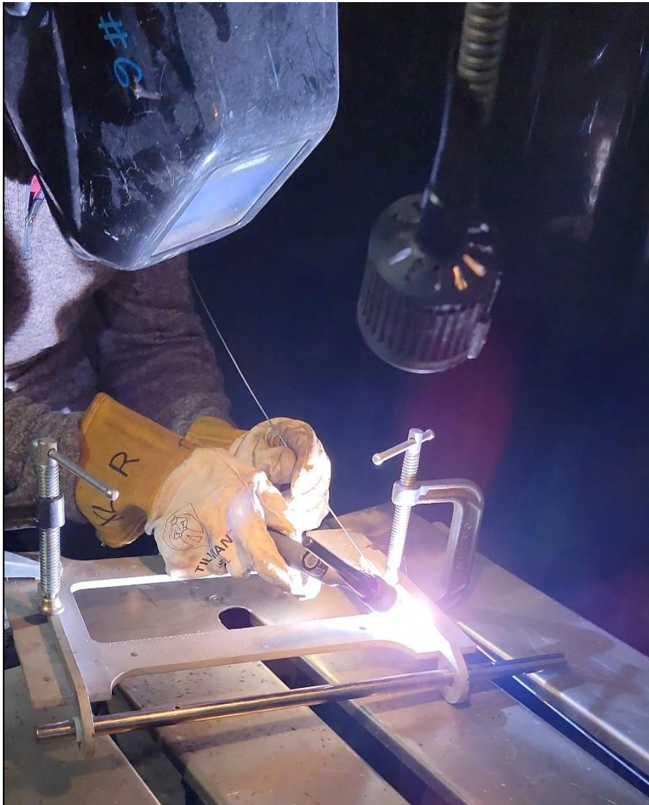
Figure 123. Tig Welding on the Seat Bottom with Supporting Bar
