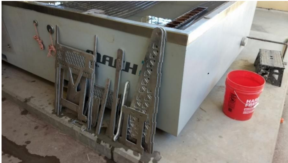
Figure 118. All parts displayed by the waterjet after removal from the plate
