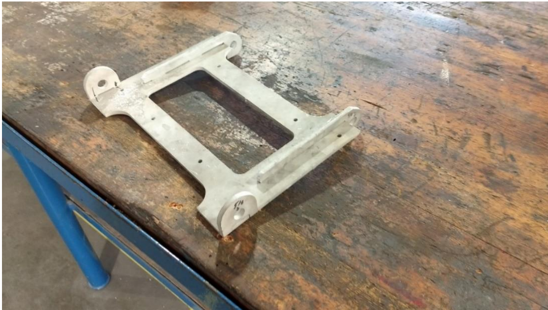
Figure 122. Seat Bottom Frame Unwelded Test Fit
