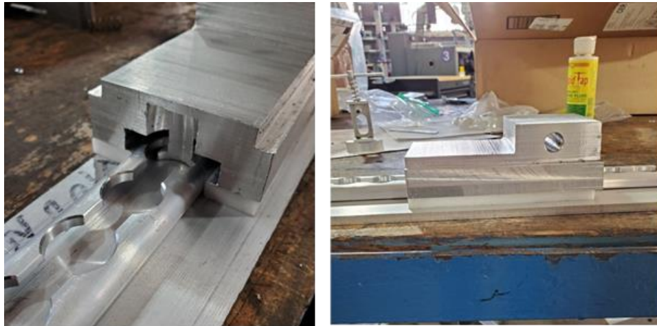
Figure 110. Completes Latch in Track Demonstrating Profile Mating
