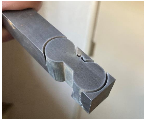
Figure 90. Double Pin Waterjet Manufacturing Error
