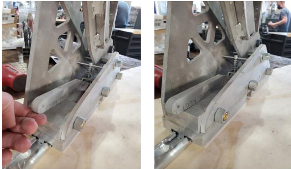
Figure 113. Attaching the CAM System to the Assembly
