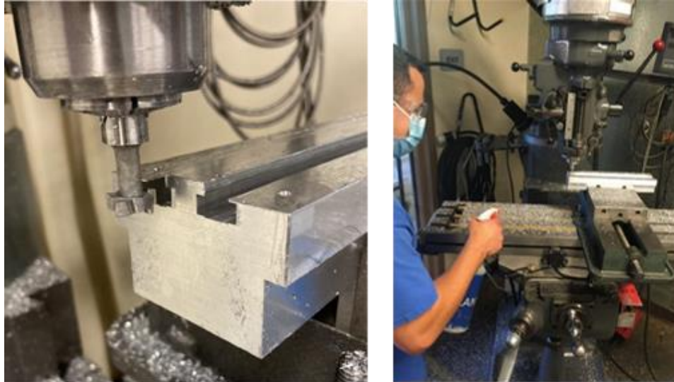
Figure 108. Milling the Mating Profile Using a T-Slot End Mill with Coolant
