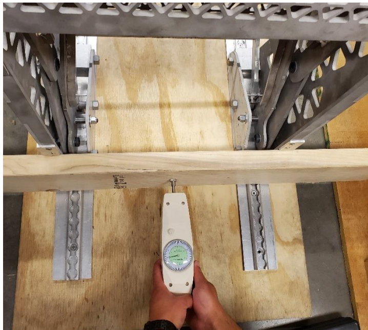
Figure 131. Testing Set up for Push Force Test
