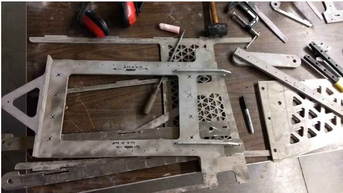
Figure 119. Holes were carefully marked to minimize the duration of the drilling operation
