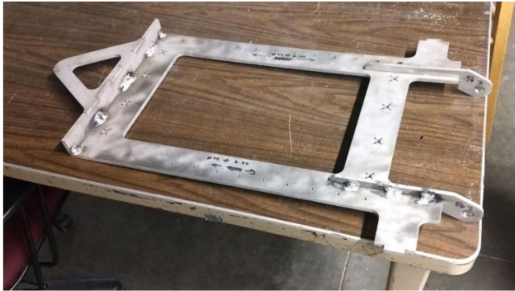
Figure 124. Completed welds on the seat back
