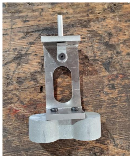
Figure 111. Complete Follower Subassembly with Double Pin
