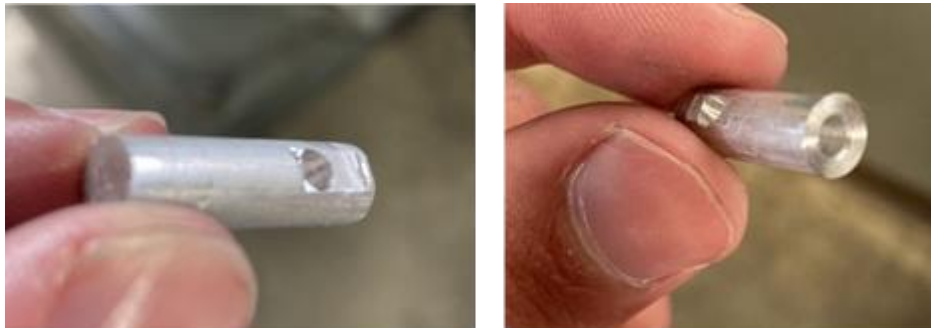
Figure 101. (Left) Female Follower Pin Showing Mounting Hole. (Right) Female Follower Pin Showing Mating Hole
