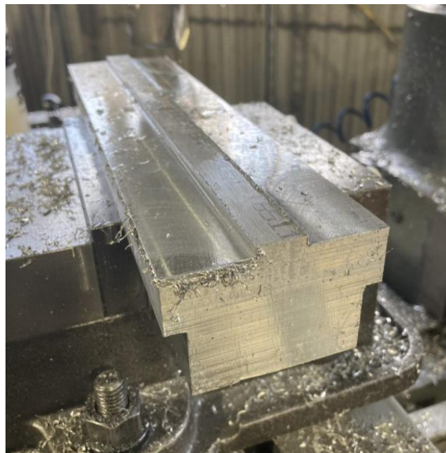
Figure 104. Initial pass for forming of track-latch profile
