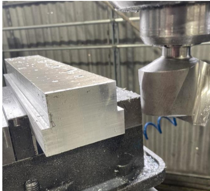
Figure 103. Initial cut from stock to rough latch shape
