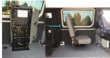
Figure 2. Freedman 3pt Double Fold-Away Seats
