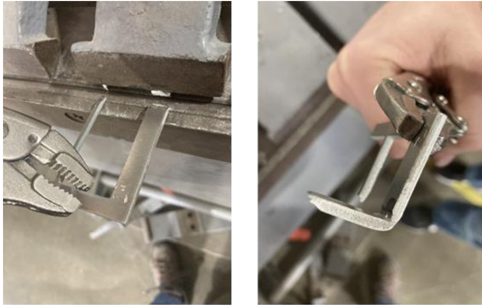
Figure 98. Test Bends of the Follower Frame
