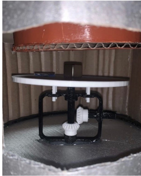
Figure 22: Magnetic Adjustment Mechanism seen through bottom window.
