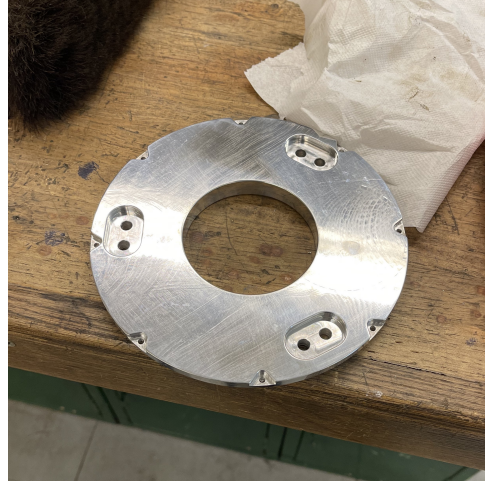
Figure 36: Final top cap part after the second procedure in the CNC. Additional hand finishing such as deburring was done as well.
