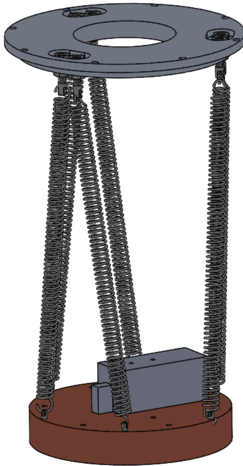
Figure 25: Assembly view of the mass-spring assembly.
