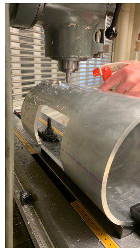
Figure 33: Aluminum housing windows being cleaned up on a manual mill using a 3/8" end mill.
