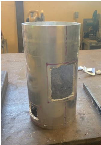
Figure 32: Aluminum cylinder after the plasma cutting procedure.
