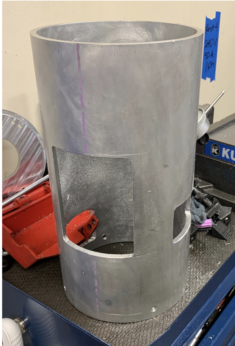
Figure 34: Aluminum housing after all manufacturing procedures have been performed.
