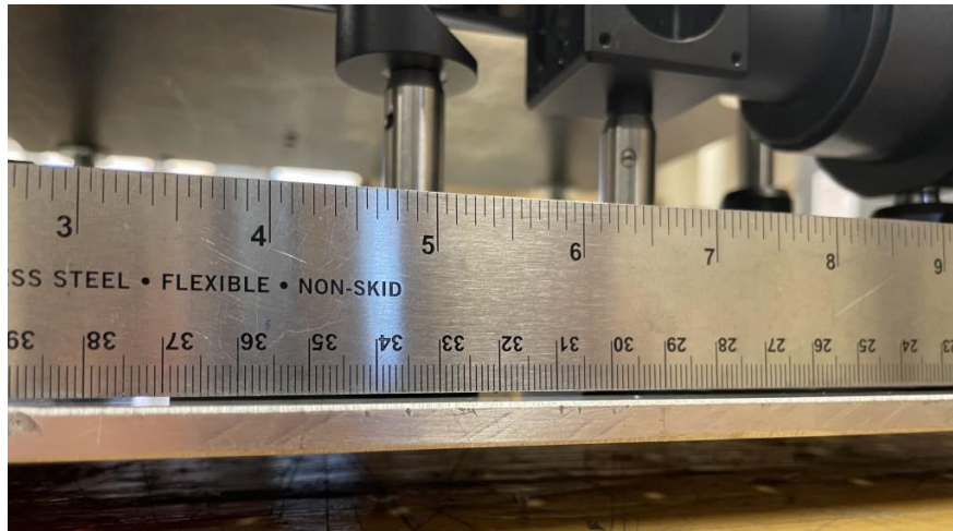
Figure 30 Deflection of un-reinforced breadboard
