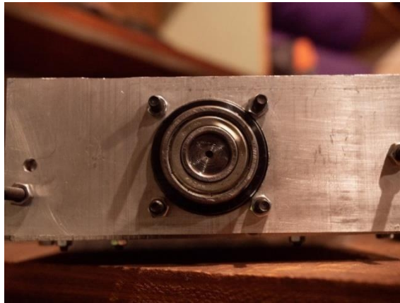
Figure 20: Ball bearing mounting configuration on the ball bearing mounting face. The ball bearing protrudes through the ball bearing mounting face and is secured with four M6 nuts and bolts.
