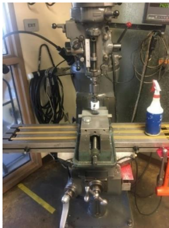
Figure 27: Cutting a starting center hole of the datum face using a hole saw.
