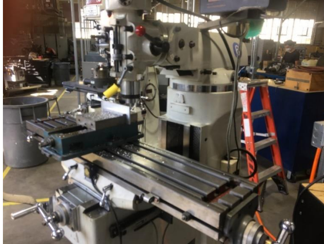
Figure 25: Flattening and squaring the edges of the motor face on the Hangar mill.
