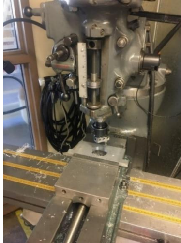
Figure 28: Using a bore bar on the Mustang 60 mill to cut the center hole of our “Datum Face”.
