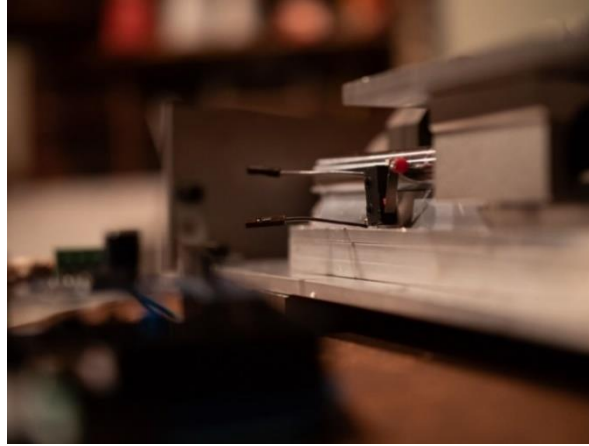
Figure 32: Limit switch mounting configuration. We mounted the limit switches at the extreme points of the table's motion on the outside of the rail and are fixed with command strips. The switches are normally closed but open the circuit upon contact with the linear bearing.
