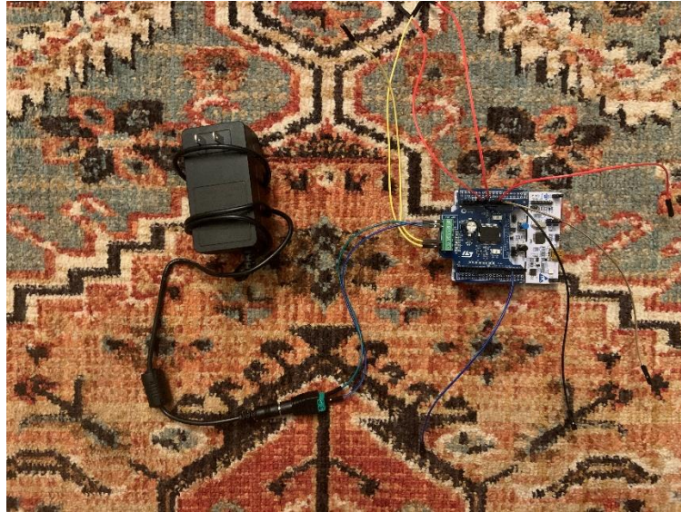
Figure 4: Motor Driver input power connected to the DC power supply to be plugged into the wall.
