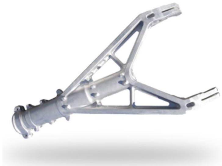
Figure 1. Landing gear shock strut produced by Weber Metals out of 7075 aluminum. The central column of the part is the thickest and poses the largest potential risk for not developing a homogenous microstructure during heat treatment. [1]
