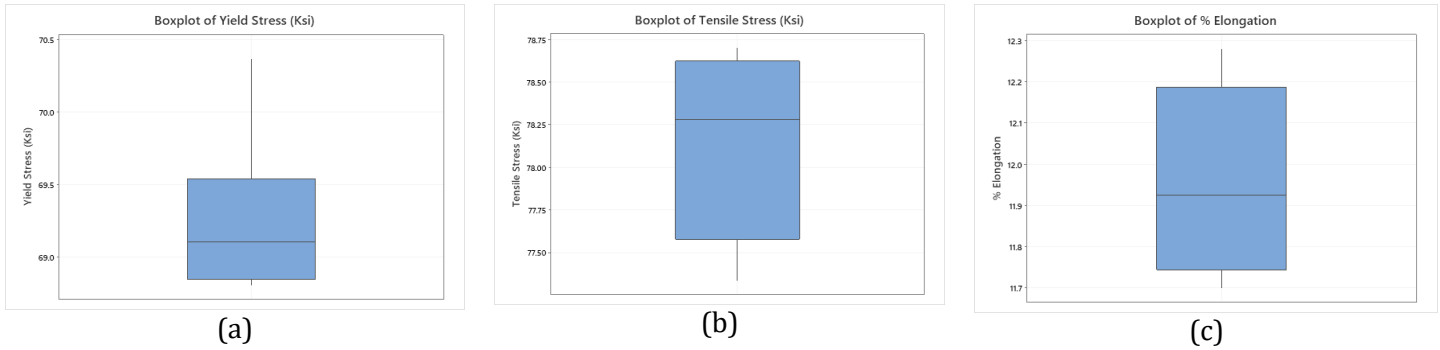
Figure 18. Box plots of the mechanical properties of the G4 heat treatment. a) is the yield strength and looks skewed, b) is the tensile strength and is fairly normally distributed c) is the percent elongation and looks normally distributed
