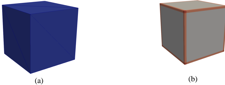
Figure 1: The geometrical STL model (a) for a simple cube and its respective porous (b) model calculated using the GJK algorithm. Threshold of the porosity is presented at the region of the computational domain where the porosity is slightly lower than unity.
