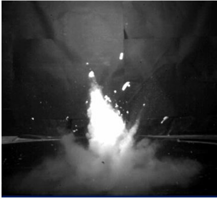
Figure 1: Talc dispersion illuminated by a powerful light source.
