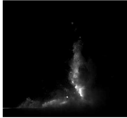
Figure 2: Talc dispersion illuminated by a laser sheet coming from the left.
