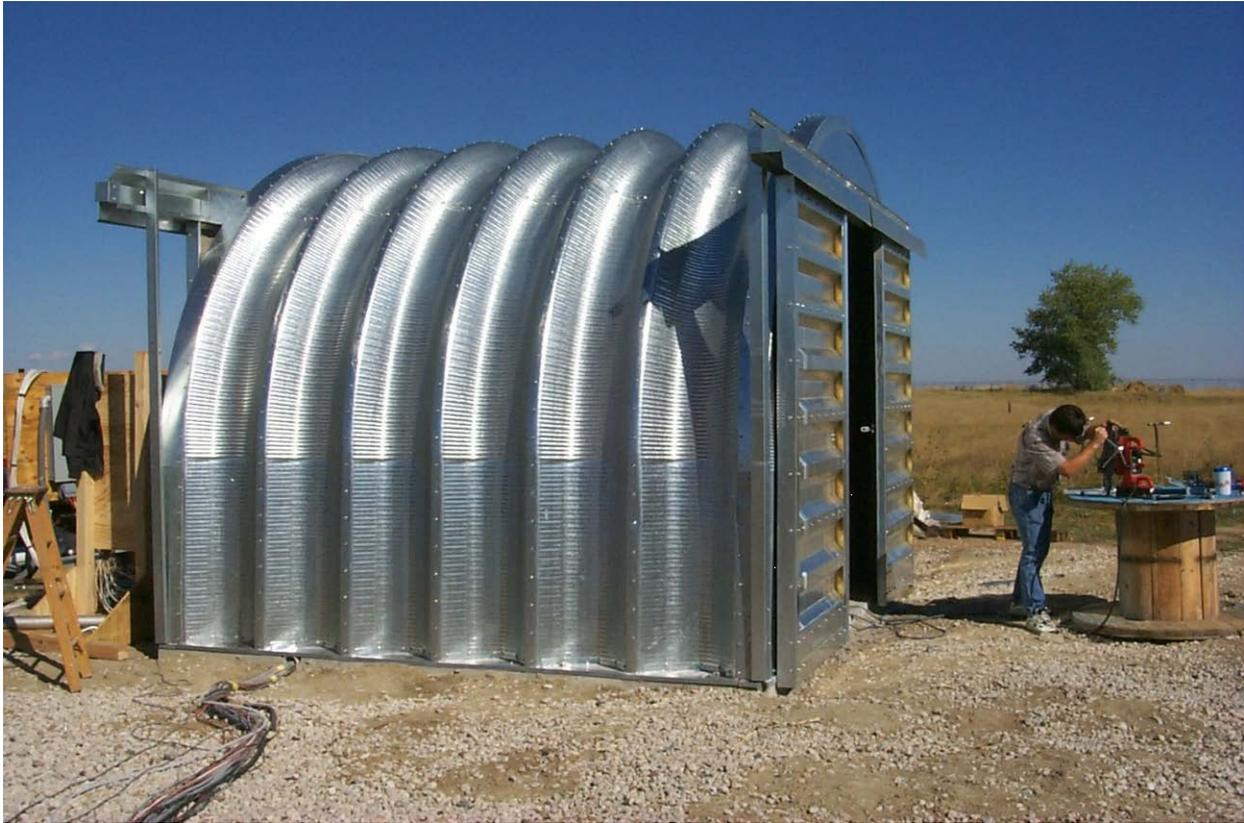
**Figure 6** Heater enclosure for the 1/4-scale set-up (Brown et al, 1999).
