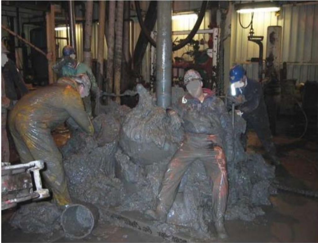
Figure 2. 2: Extreme case of Gumbo shale instability- flow to the surface due to incompatible mud type with the formation [49]
