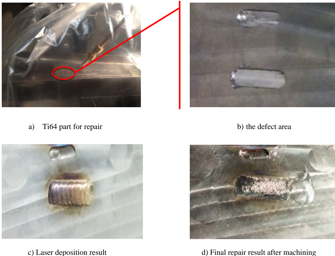
Figure 6: The result of deposition and machining for Ti64 part repair
